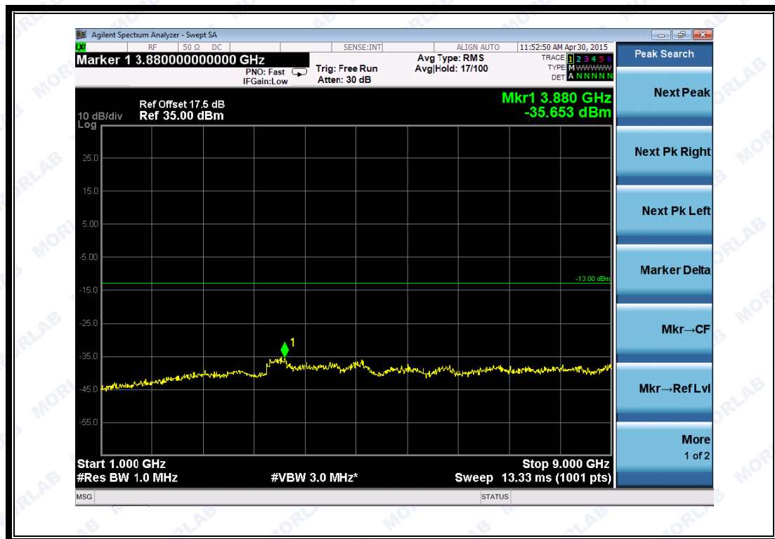
(Plot I2.1: HSUPA 850MHz Channel = 4175, 1GHz to 9GHz)
