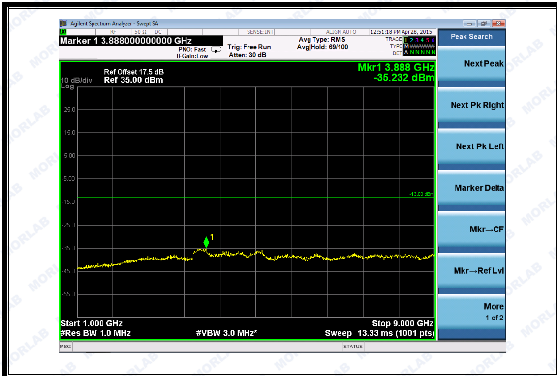
(Plot E1.1: WCDMA850MHz Channel = 4132, 1GHz to 9GHz)
