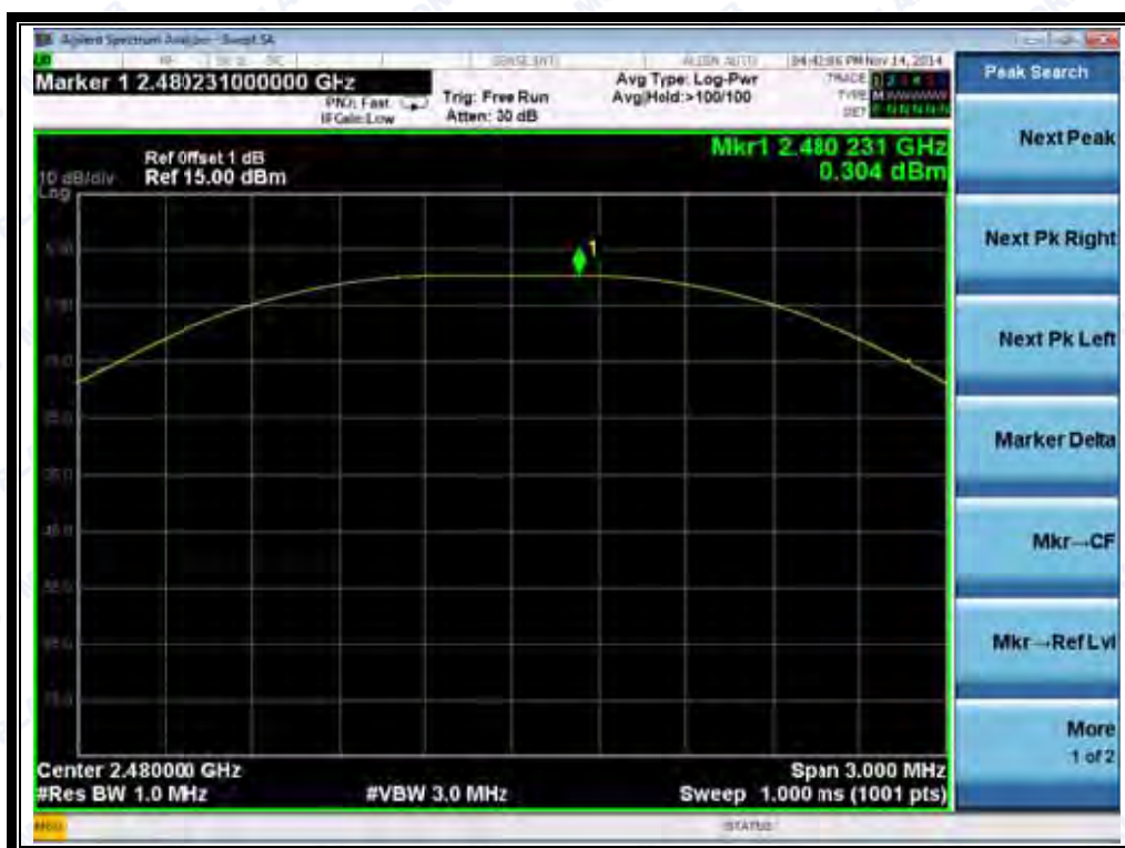
(Plot C: Channel 39: 2480MHz)
