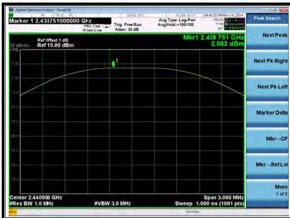
(Plot B: Channel 19: 2440MHz)
