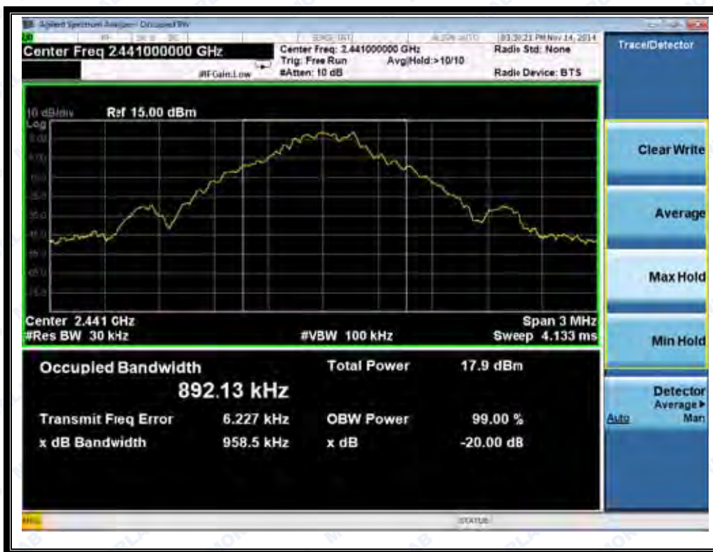
(Plot B: Channel = 2441 @ GFSK)
