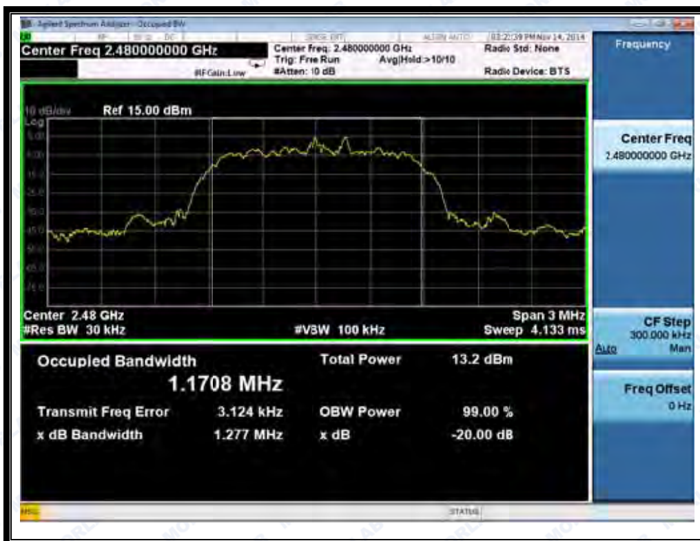
(Plot F: Channel = 2480 @ \pi/4 -DQPSK)
