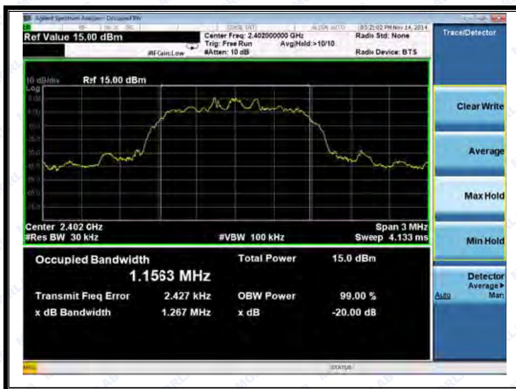
(Plot D: Channel = 2402 @ \pi/4 -DQPSK)
