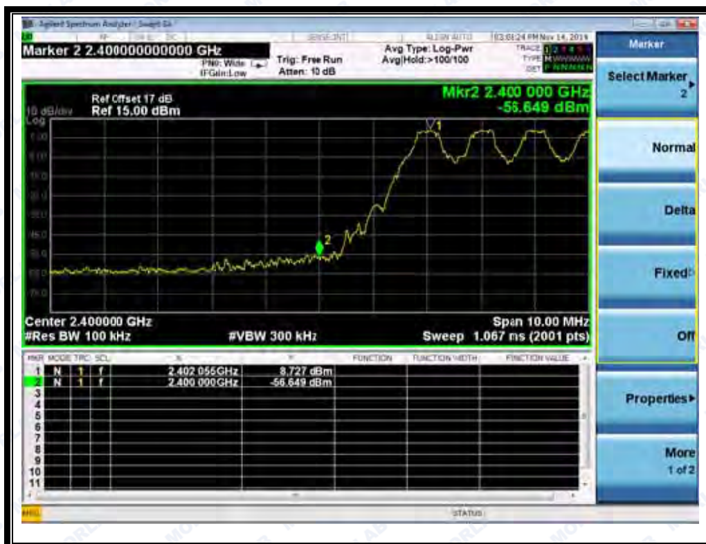
(Channel = 0, Band edge with hopping on @ GFSK Mode)
