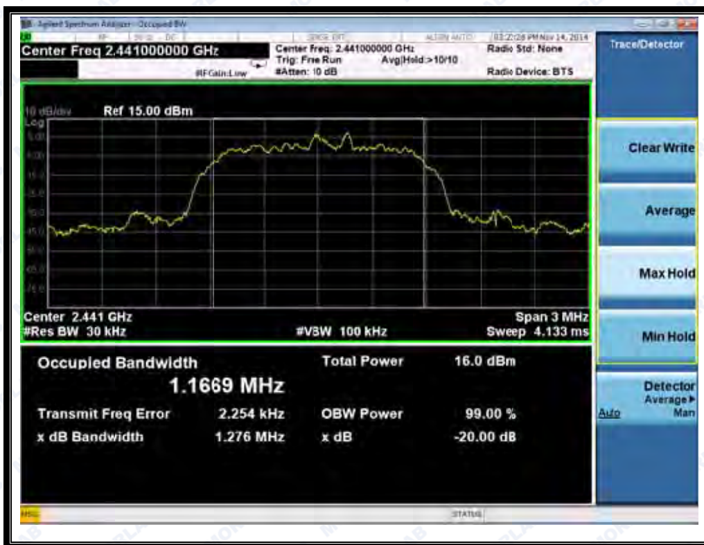
(Plot E: Channel = 2441 @ \pi/4 -DQPSK)
