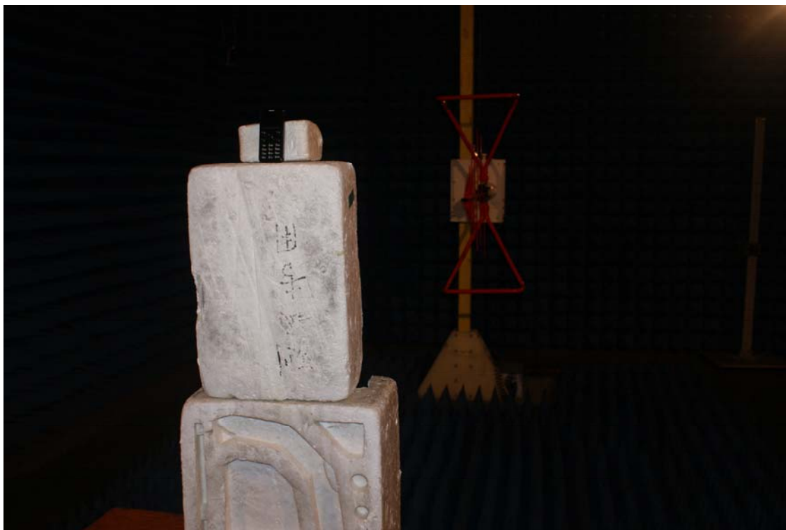
RADIATED EMISSION TEST SETUP
