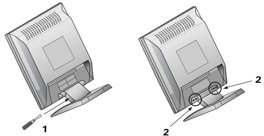
1. Detach the rear cover of the stand with a screwdriver.
