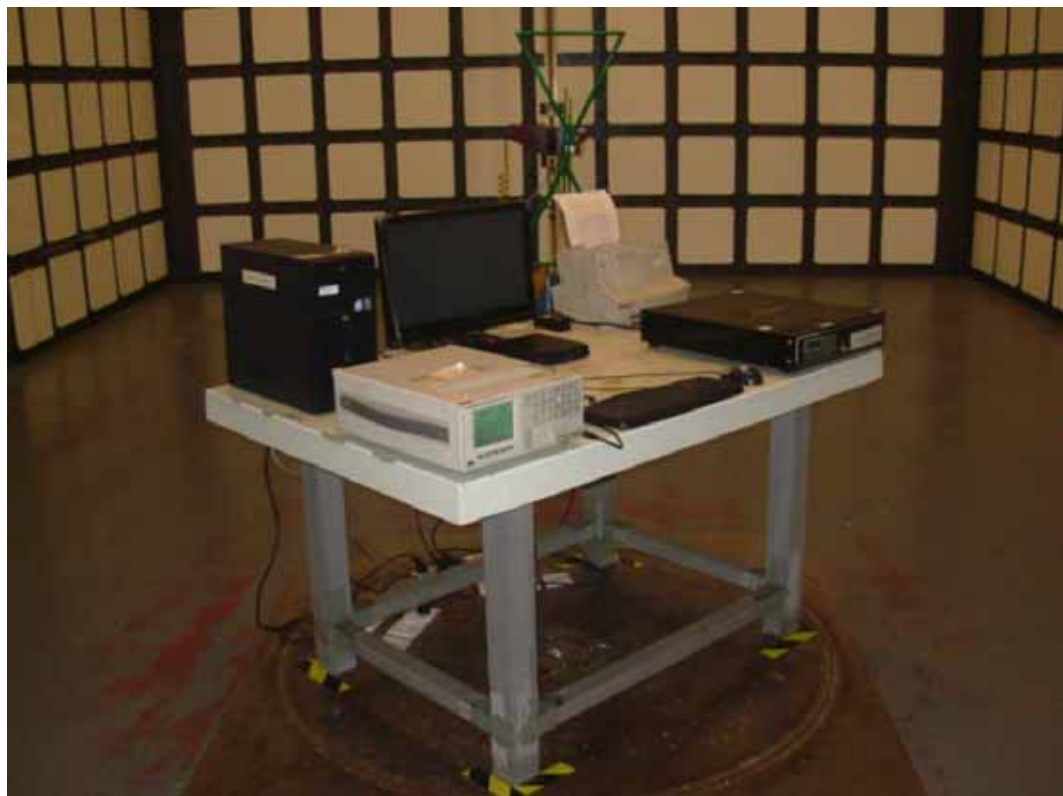
SETUP WITH MAXIMUM DETECTED EMISSION AT VERTICAL POLARIZATION (D-SUB 1366*768@60Hz)
