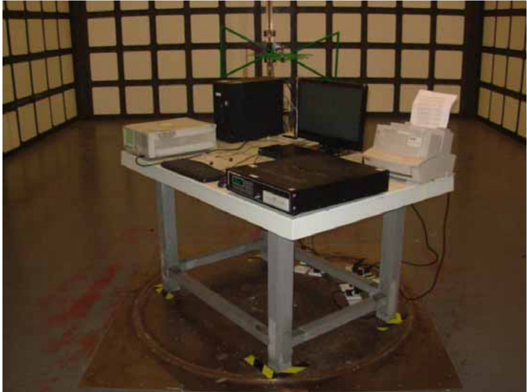
SETUP WITH MAXIMUM DETECTED EMISSION AT HORIZONTAL POLARIZATION (D-SUB 1366*768@60Hz)
