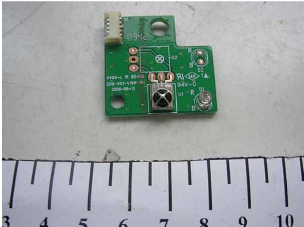
FIGURE 8 LCD TV (M/N: ELETT221) LED BOARD (COMPONENT SIDE)
