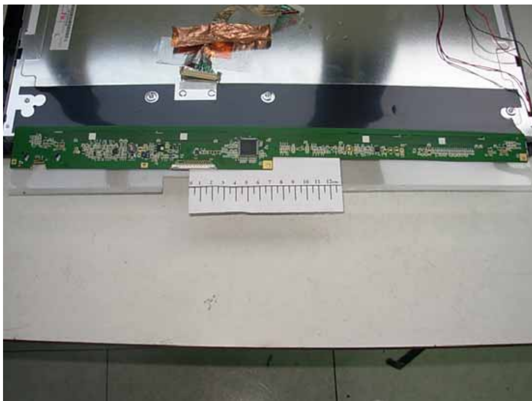
FIGURE 10 LCD TV (M/N: ELETT221) LED PANEL CONTROL BOARD (COMPONENT SIDE)
