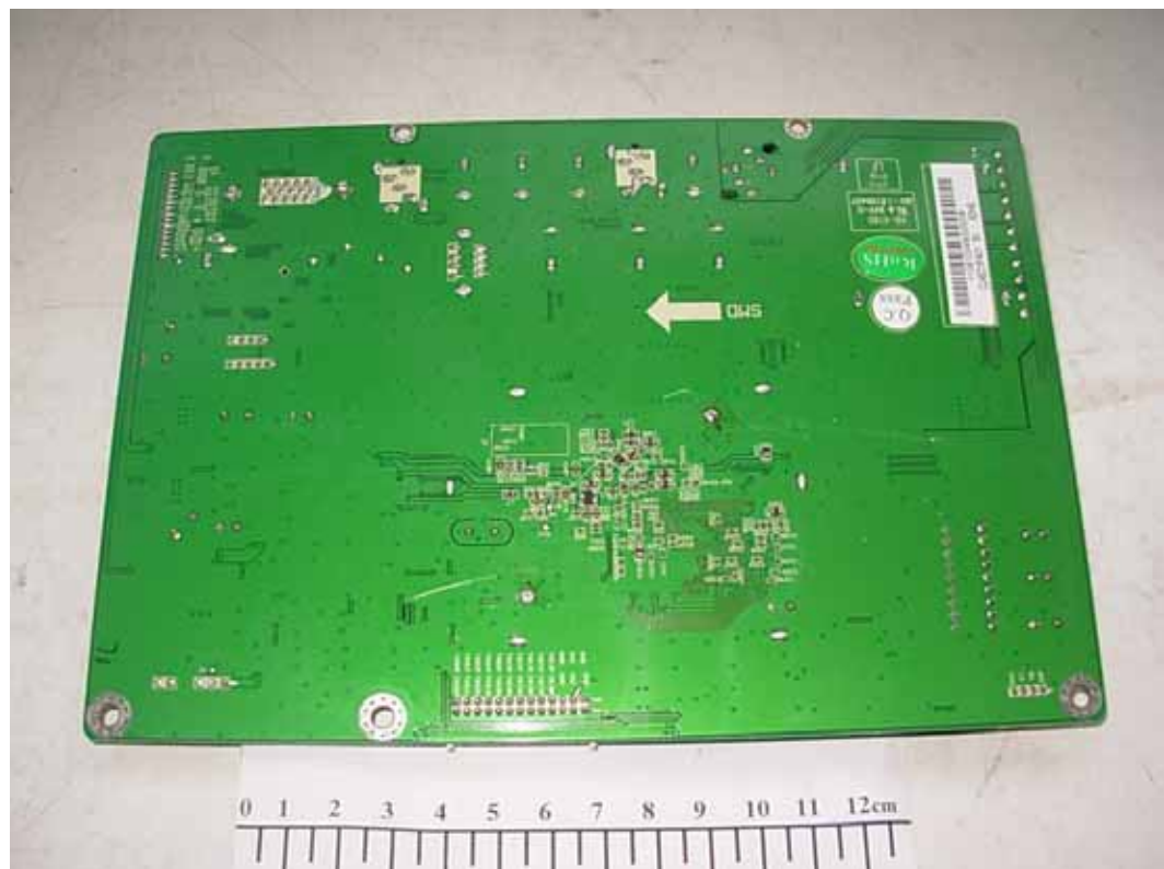
FIGURE 3 LCD TV (M/N: ELETT221) MAIN BOARD (SOLDERED SIDE)
