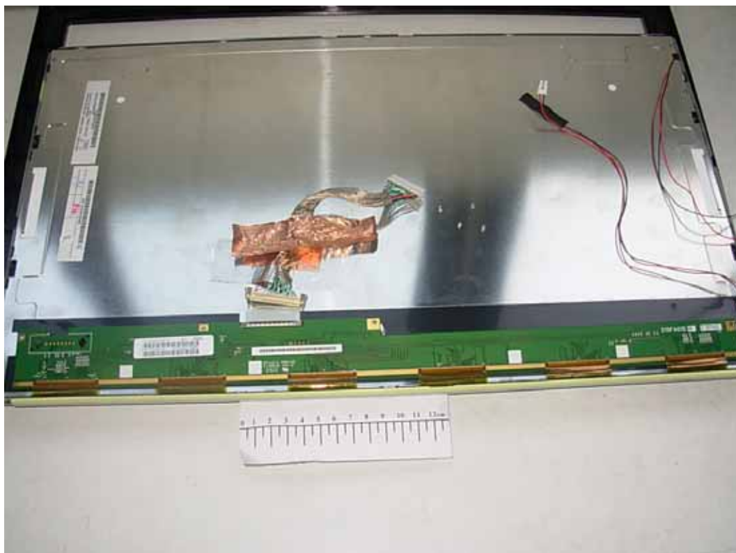
FIGURE 11 LCD TV (M/N: ELETT221) LED PANEL CONTROL BOARD (SOLDERED SIDE)
