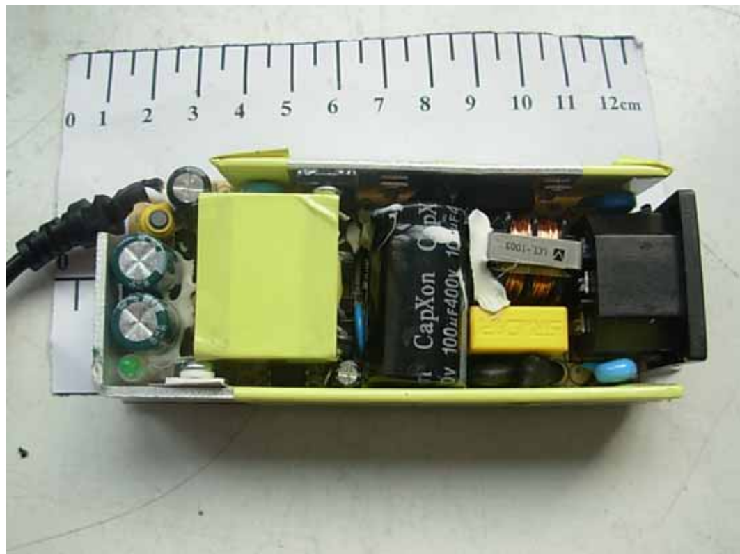
FIGURE 8 LCD TV (M/N: ELETT221) ADAPTER (POWER BOARD – COMPONENT SIDE)
