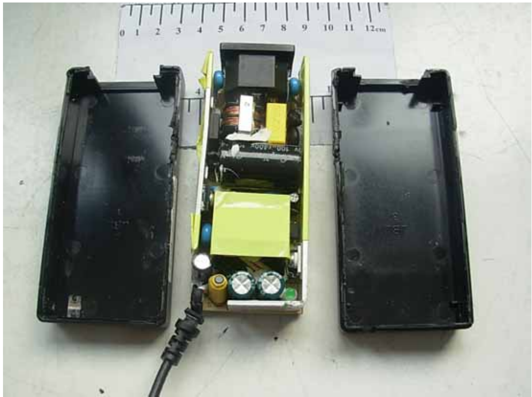
FIGURE 7 LCD TV (M/N: ELETT221) ADAPTER (COVER REMOVED)
