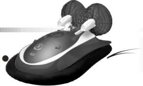
⑤ Connect the battery switch on the hovercraft, start up the high pressure motor inside the ship to inflate the hood of the hovercraft, and enter the operable status.
