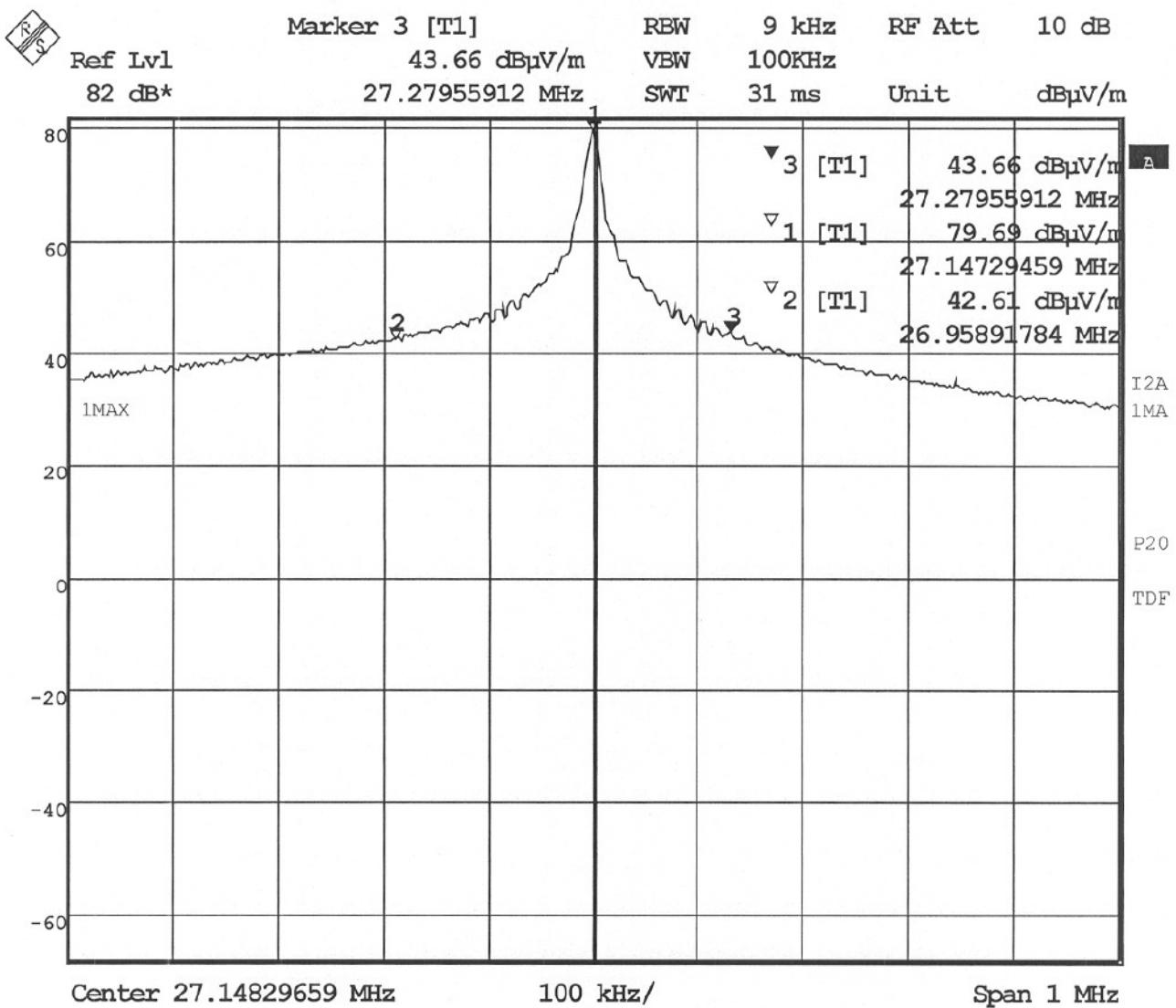
**Result:** The field strength of any emission within the operation band did not exceed 80dB( $\mu$  V/m) for average value or 100 dB( $\mu$  V/m) for peak value.
