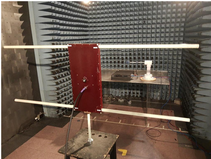
Figure 4: Radiated Immunity - Test Setup for 1MHz
