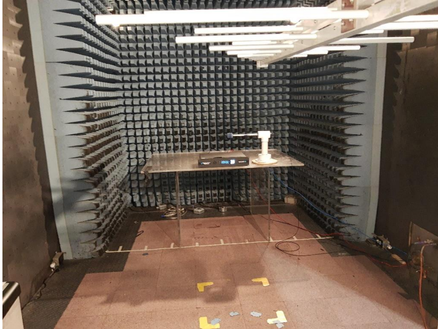
Figure 1: Radiated Immunity - Test Setup for 108MHz
