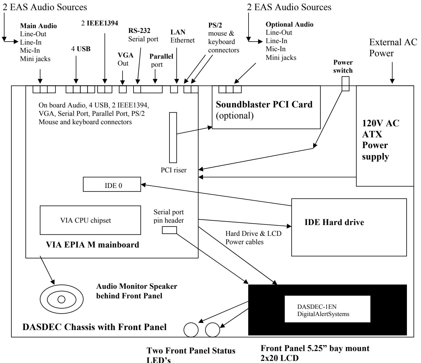
The DASDEC-1EN EAS Encoder/Decoder is a an embedded PC motherboard device that is completely software driven. It is controlled over a LAN or by a desktop browser interface using the built in VGA output, mouse, and keyboard. Two external mono EAS audio sources (from a radio, EAS encoder, soundcard, etc) can be connected to each Audio Line-Input to decode two EAS sources per input. Any audio output can be selected for EAS encoded audio output.
