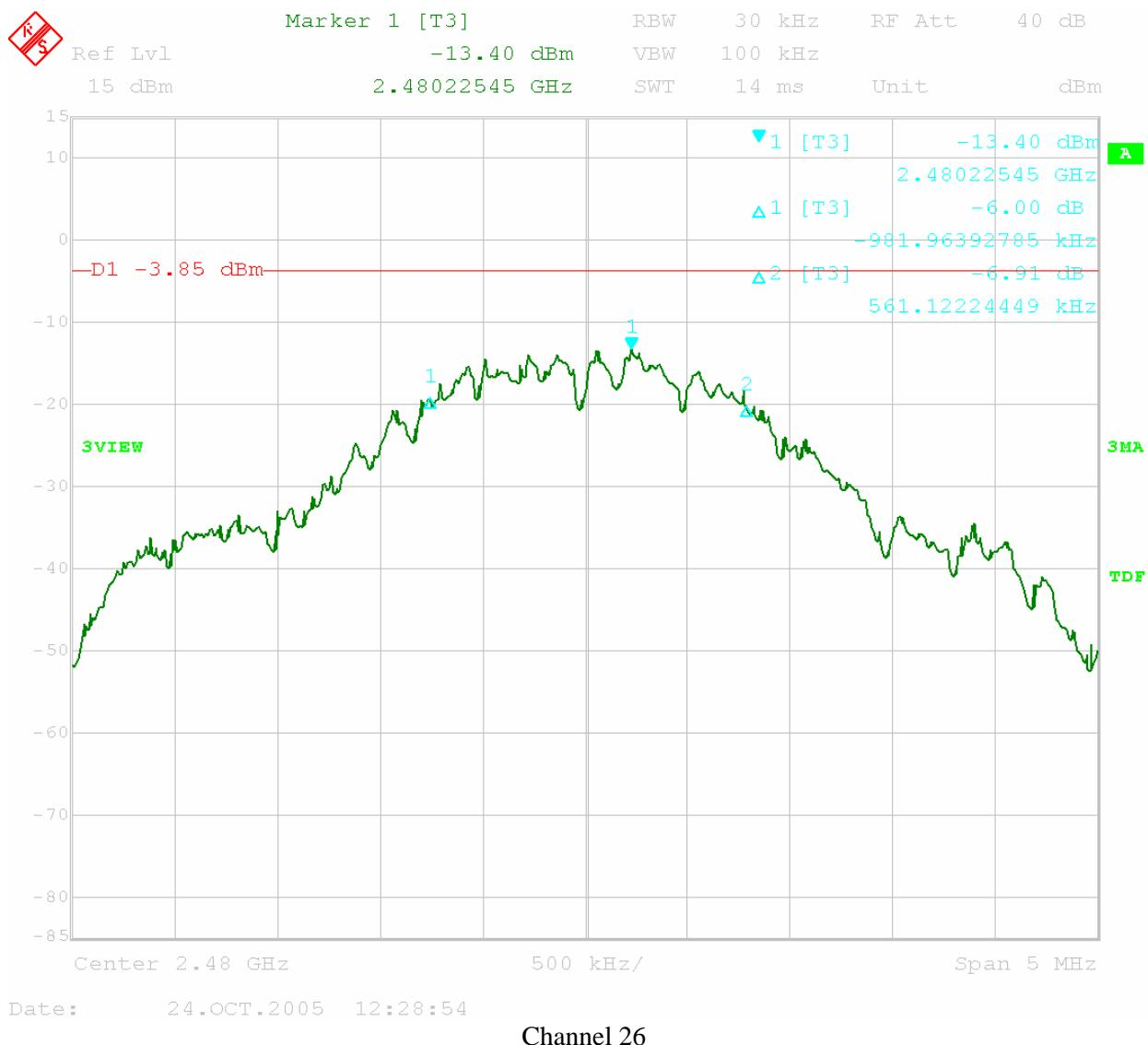
**Test Results:** Pass**Test Standard:** FCC 15.247(b)(3-5)**Test:** Maximum Peak Conducted Output Power and Human RF Exposure**Performance Criterion:** The output power must not exceed 1 Watt (30 dBm) and 36 dBm EIRP. The human RF Exposure limit is 1 mW/cm<sup>2</sup>.**Test Date:** 10/24/2005**Engineer Initials:** NNA**Date:** 10/27/05**Test Engineer:** Nicholas Abbondante**Reviewer Initials:** rwj**Date:** 10-28-2005**Test Equipment Used:**
