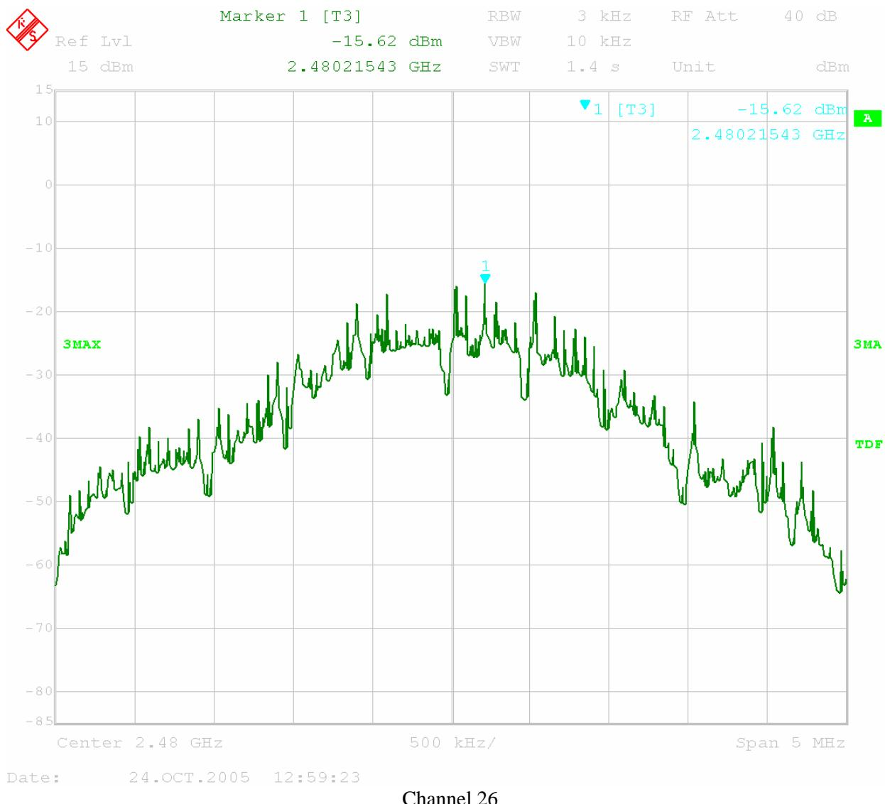
**Test Results: Pass****Test Standard:** FCC 15.215**Test:** Band Edge Compliance**Performance Criterion:** The fundamental frequency must stay within the assigned frequency band.
