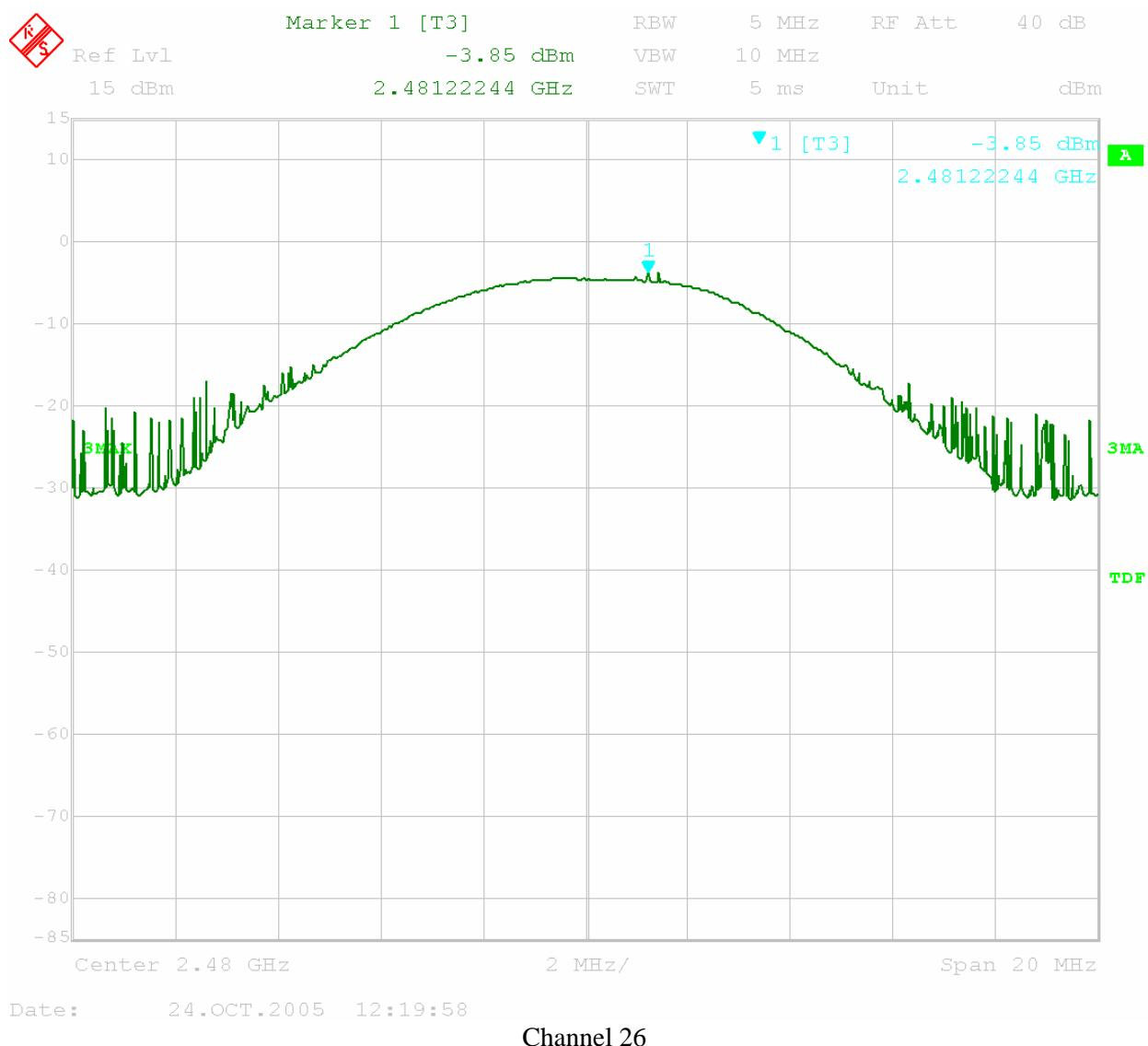
**Test Results:** Pass**Test Standard:** RSS-210 A8.5**Test:** Antenna Port Conducted Spurious Emissions**Performance Criterion:** The spurious emissions must be attenuated below the level of the fundamental by at least 20 dBc.
