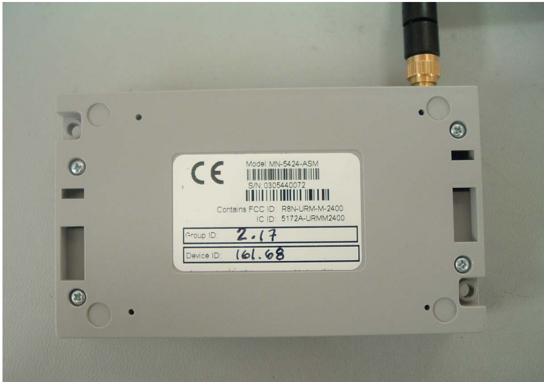
MN-5424 Labeling Area
