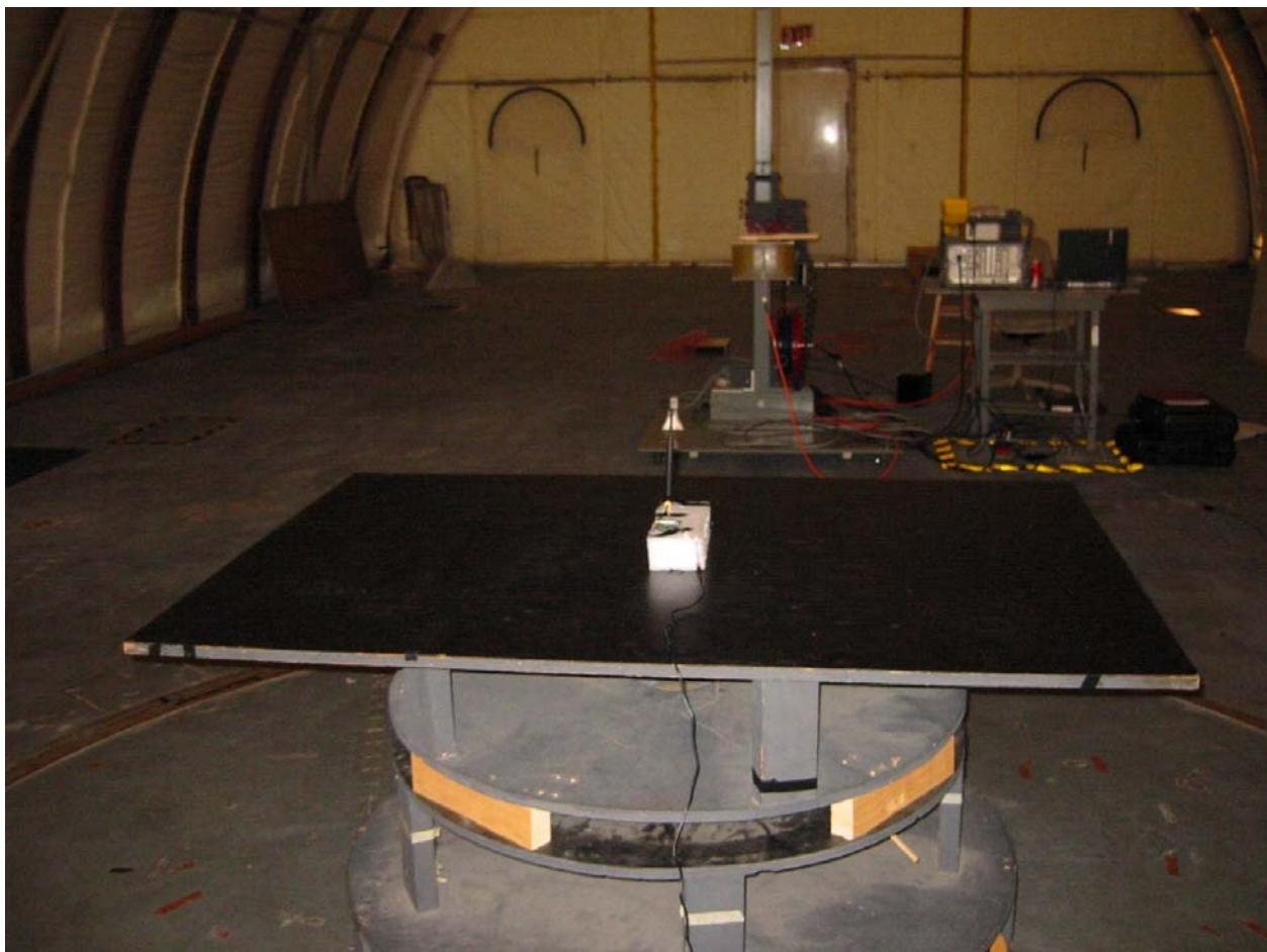
**Test Results: Pass****Test Standard:** FCC 15.247(e)**Test:** Peak Power Spectral Density**Performance Criterion:** The peak power spectral density must not exceed 8 dBm / 3 kHz.**Test Date:** 10/14/2005**Engineer Initials:** nwa**Date:** 10/25/05**Test Engineer:** Nicholas Abbondante**Reviewer Initials:** PWG**Date:** 10-25-2005**Test Equipment Used:**
