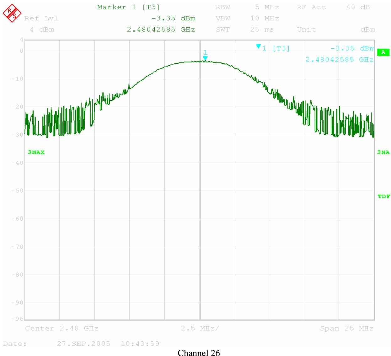
**Test Results: Pass****Test Standard:** FCC 15.209, 15.247(d)**Test:** Antenna Port Conducted Spurious Emissions**Performance Criterion:** The spurious emissions must be attenuated below the level of the fundamental by at least 20 dBc.**Test Date:** 9/27/2005**Test Engineer:** Nicholas Abbondante**Engineer Initials:** nna**Reviewer Initials:** RWJ**Date:** 10/11/05**Date:** 10-13-05**Test Equipment Used:**
