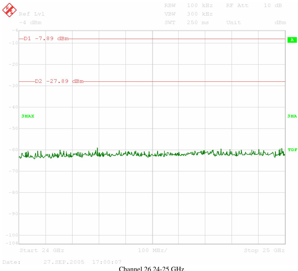
**Test Results:** Pass**Test Standard:** FCC 15.205, 15.209, 15.247(d)**Test:** Radiated Spurious Emissions**Performance Criterion:** The spurious emissions must be attenuated below the level of the fundamental by at least 20 dBc. Emissions which fall in the restricted bands must meet the general limits of 15.209.**Software:**
