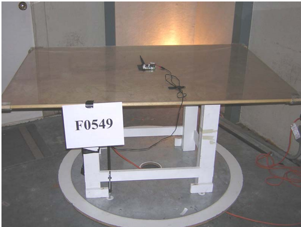
Fundamental and Harmonic Emissions, Bandwidth, and Voltage Variations
