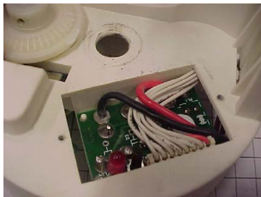
PHOTO N° 4 – INTERNAL VIEW: RECEIVER MODULE AND ANTENNA
