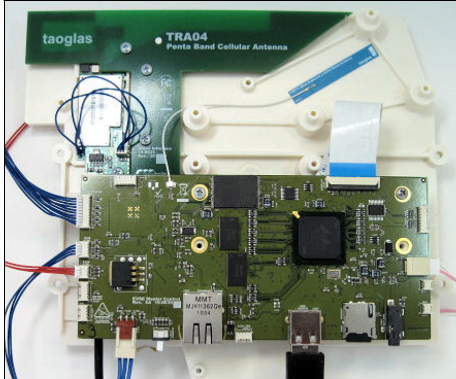
Unigen Module Mounted with New Antenna
