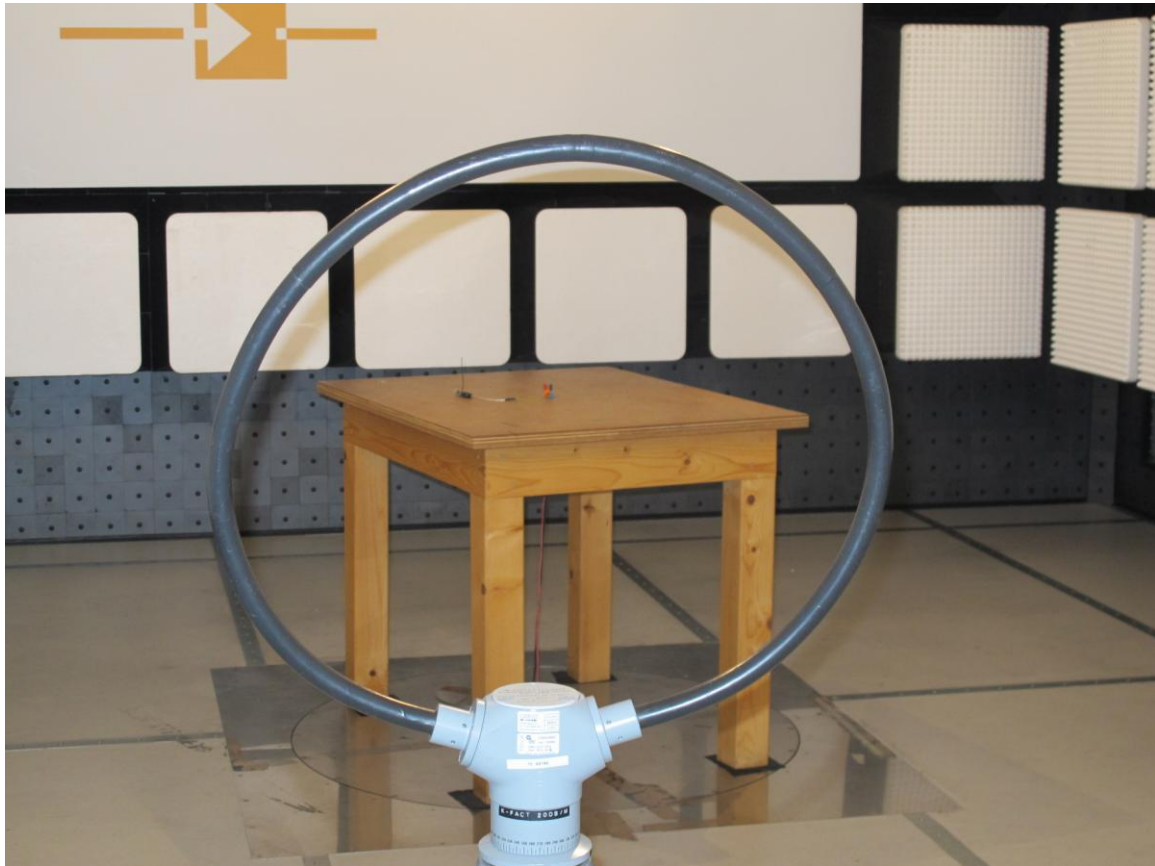
Photograph 1: Radiated emissions test set up, 0.15 – 30 MHz
