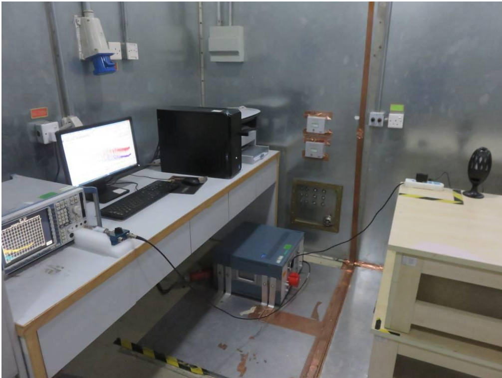
FCC RADIATED EMISSION TEST SETUP
