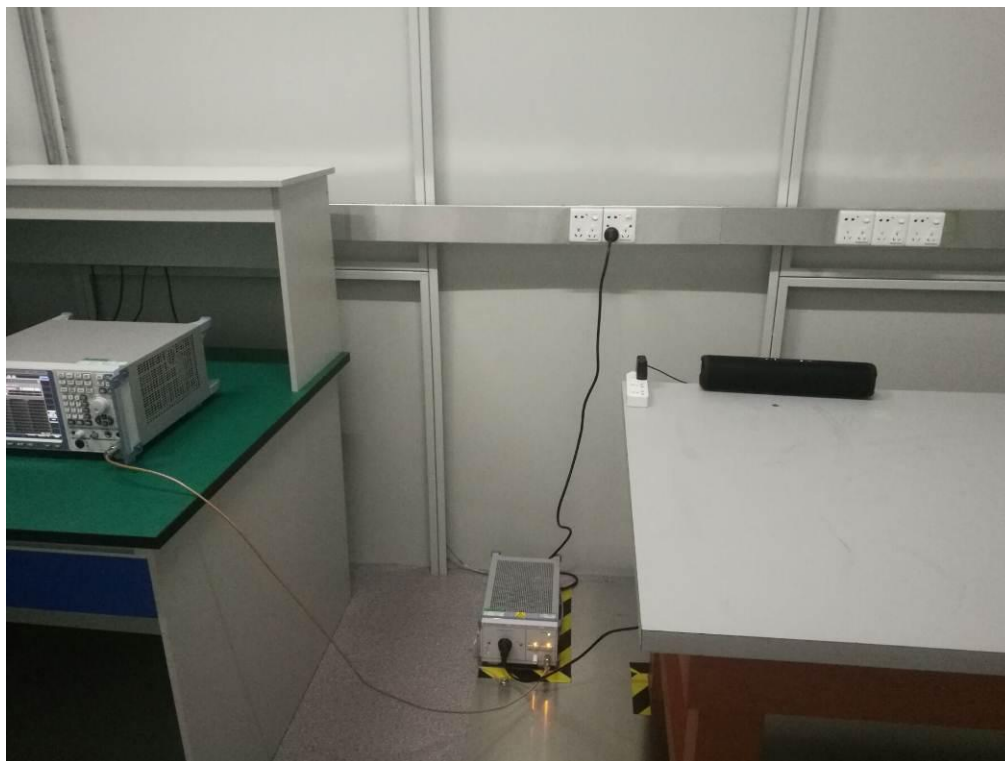
FCC RADIATED EMISSION TEST SETUP
