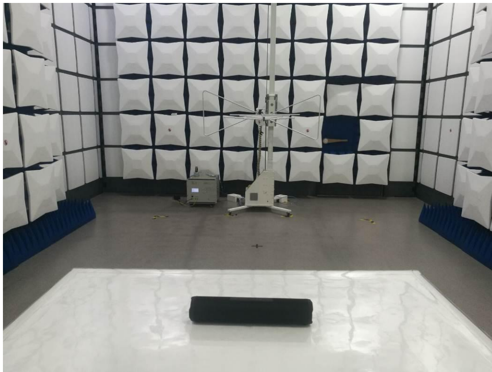
FCC RADIATED EMISSION TEST SETUP
