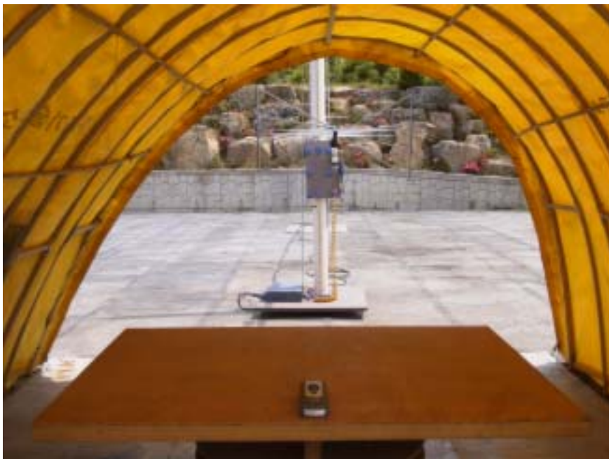
Photograph 1 : Setup for radiated Emissions
