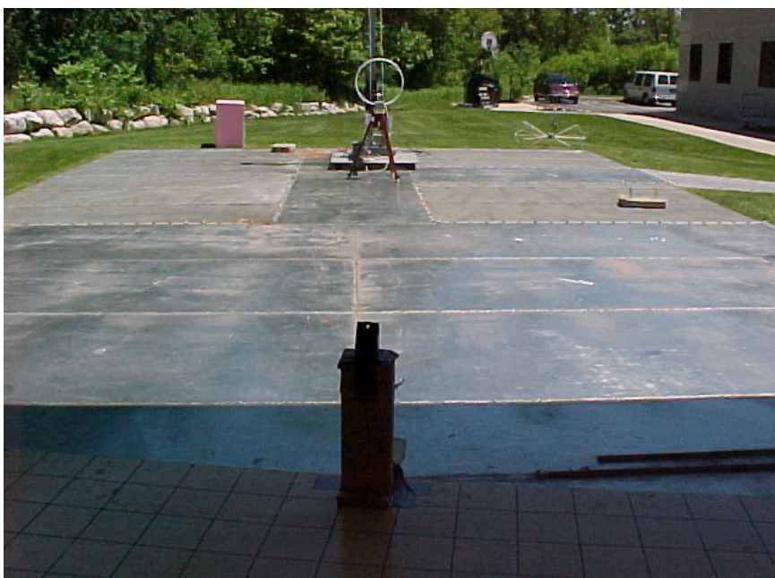
Views of the EUT during Radiated Emissions testing on the 10 Meter FCC listed OATS.
