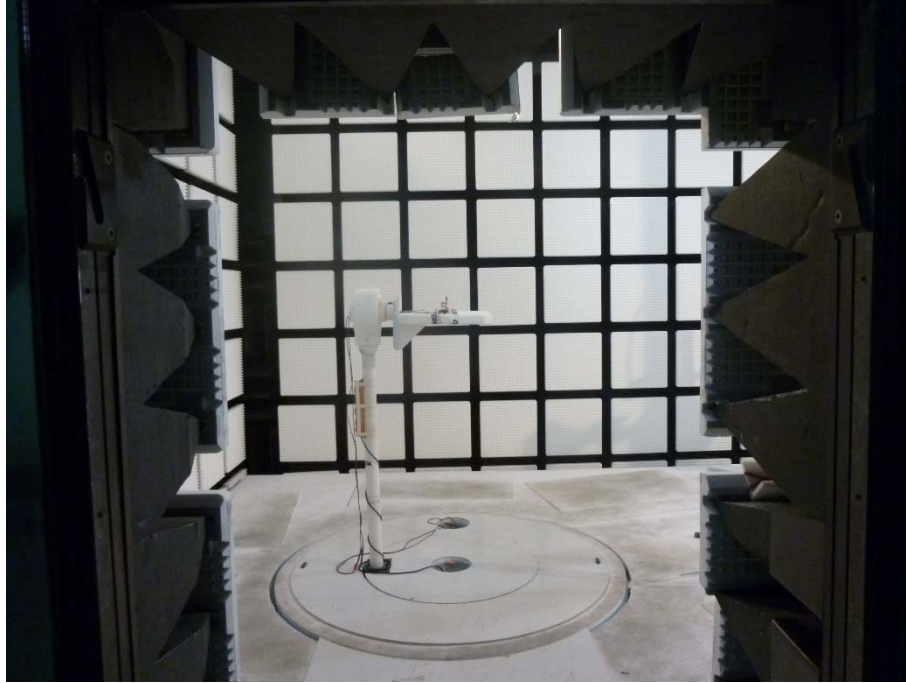
Photo 1: EUT at the anechoic chamber
