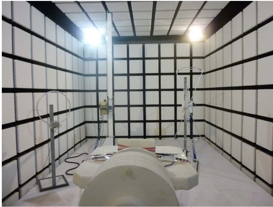
Photo 3: EUT at the anechoic chamber
