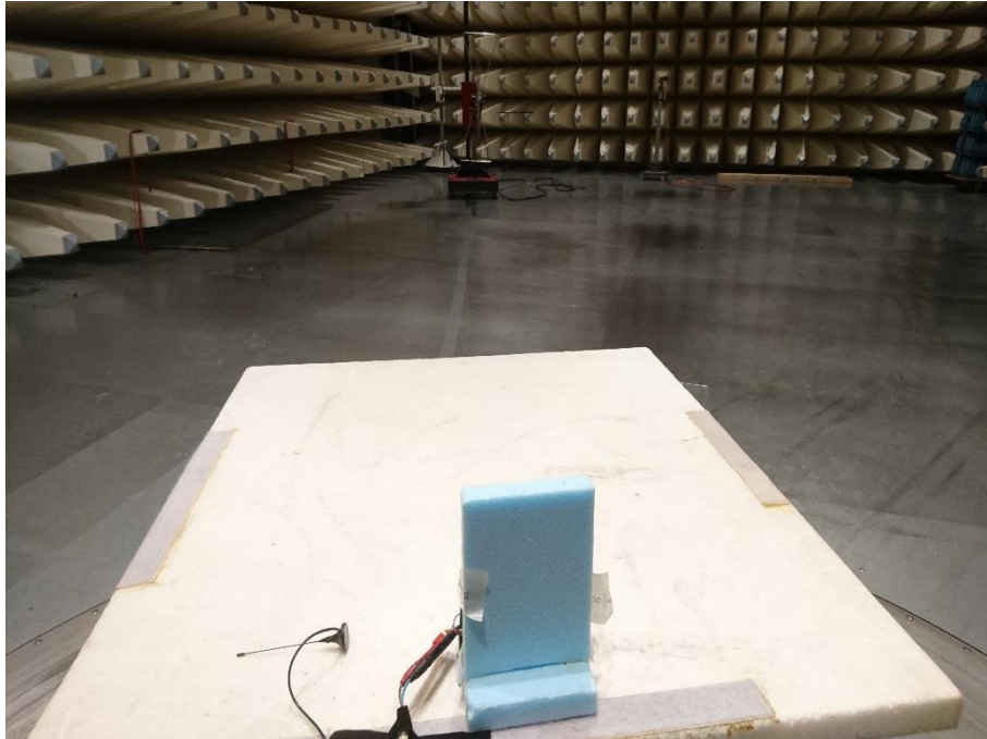
Photo 11: EUT at the semi-anechoic chamber
