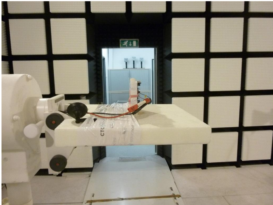
Photo 4: EUT at the anechoic chamber
