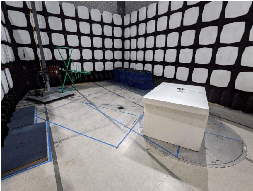
Figure 2 – Test Set up - Radiated Emissions <1 GHz
