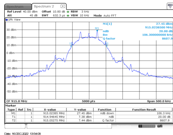
Figure 2.8.6-2: Mode 1 – 20 dB BW – MCH – 50 kbps
