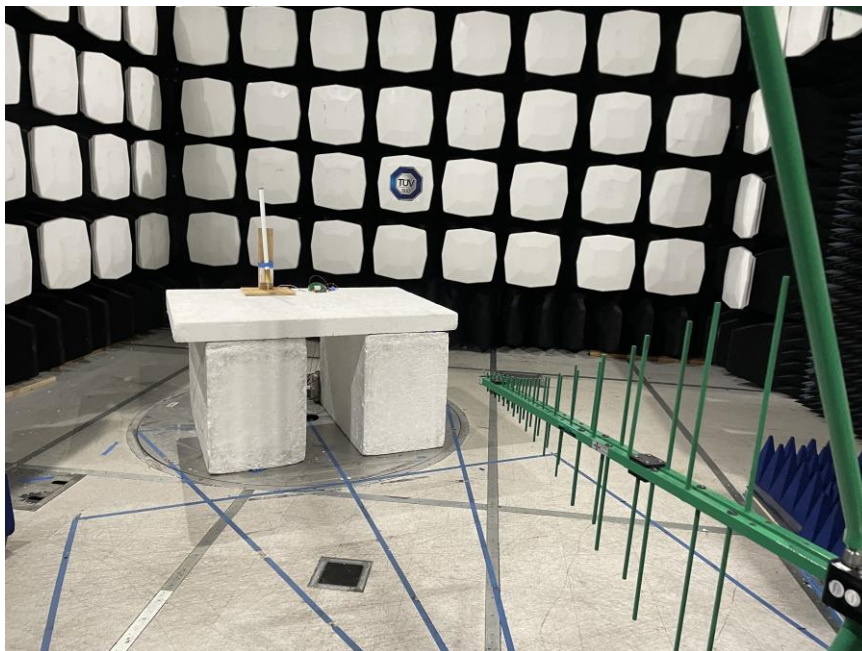
Figure3 – Test Set up - Radiated Emissions <1 GHz – Dipole Antenna
