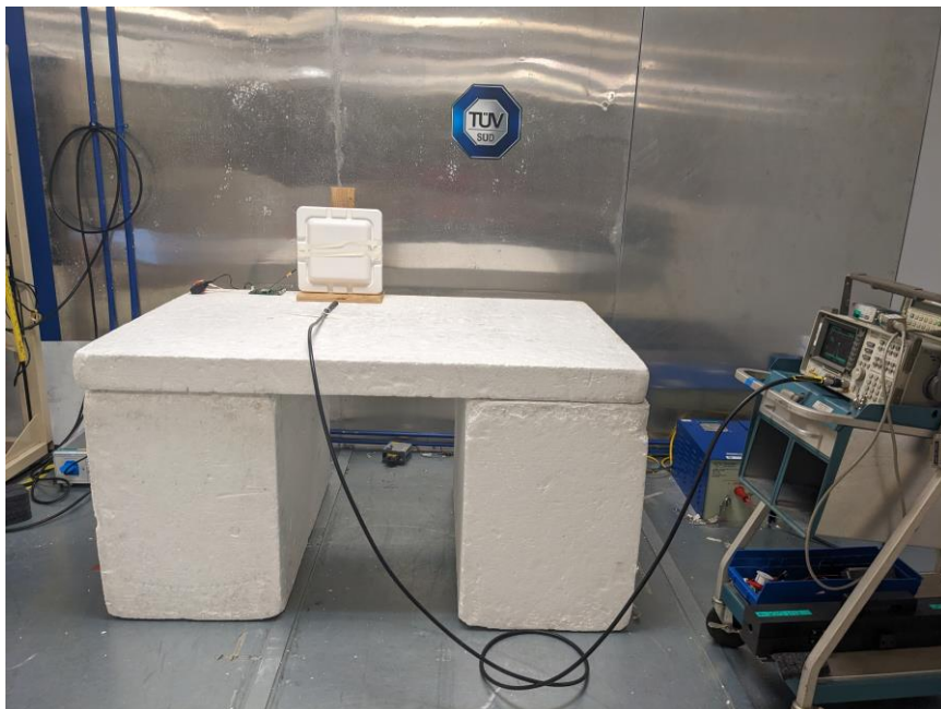
Figure8 – Test Set up – Conducted Emissions – Sector Antenna
