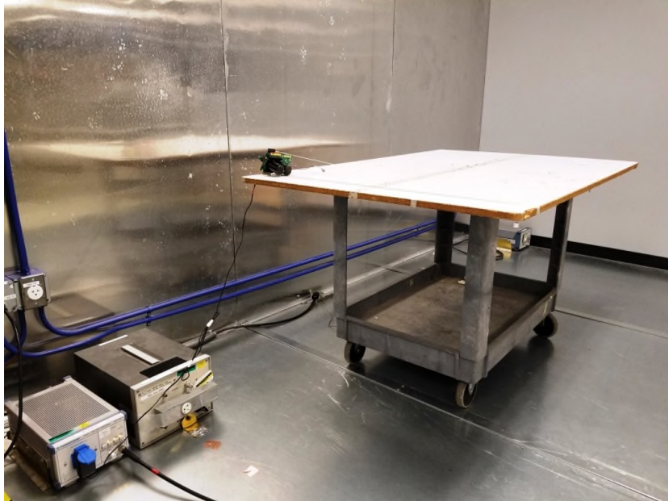
Figure 5: Equipment Under Test – AC Conducted Emissions
