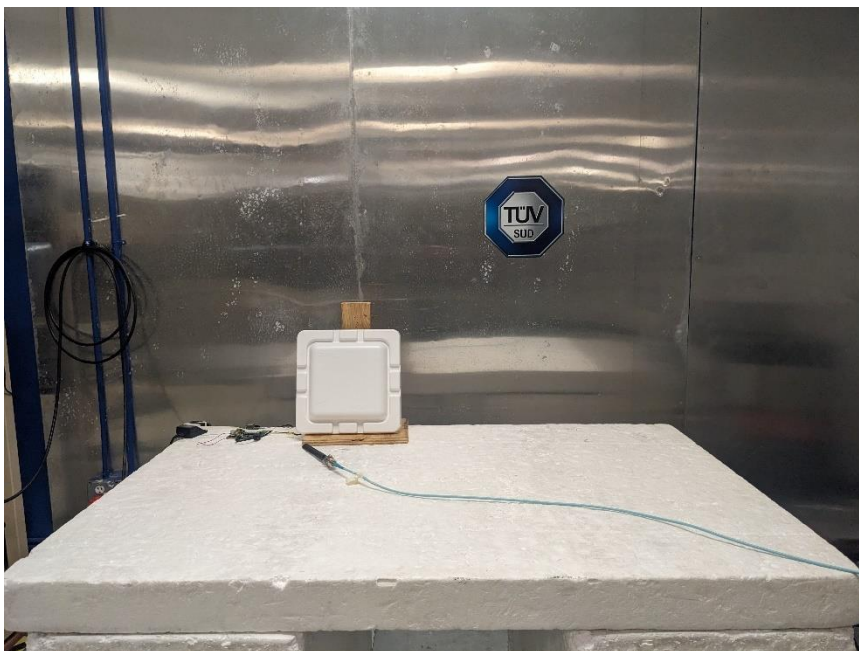
Figure 14 – Test Set up – Conducted Emissions – Sector Antenna
