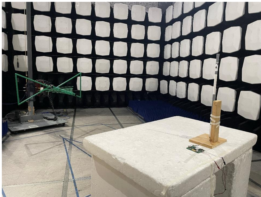
Figure 6 – Test Set up Rear View - Radiated Emissions <1 GHz – Dipole Antenna
