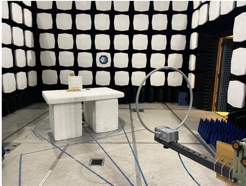
Figure 3 – Test Set up Front View - Radiated Emissions <30 MHz – Sector Antenna
