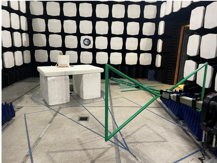
Figure 7 – Test Set up Front View- Radiated Emissions <1 GHz – Sector Antenna
