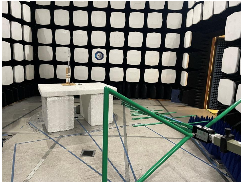
Figure 5 – Test Set up Front View - Radiated Emissions <1 GHz – Dipole Antenna
