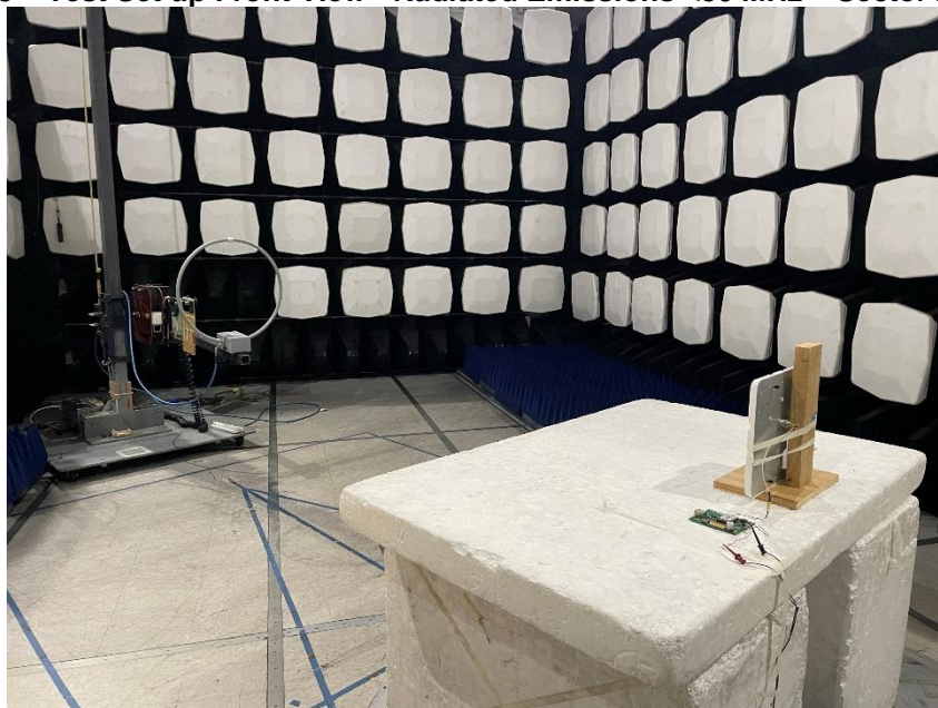
Figure 4 – Test Set up Rear View - Radiated Emissions <30 MHz – Sector Antenna
