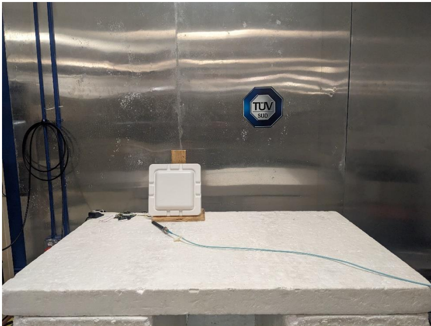
Figure 14 – Test Set up – Conducted Emissions – Sector Antenna
