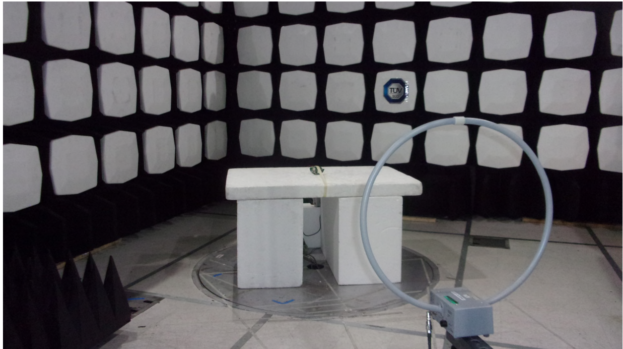
Figure 1: Equipment Under Test – Radiated Emissions <30MHz
