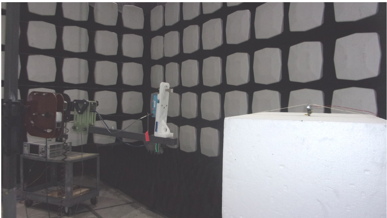
Figure 8: Equipment Under Test – Radiated Emissions >18GHz
