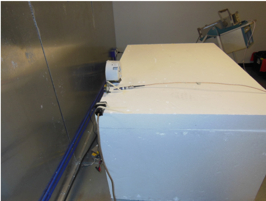
Figure 9: Equipment Under Test – AC Conducted Emissions
