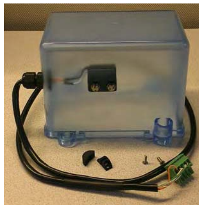
Figure 1 - 11. Solid State Pulser Index Cover With Magnet Wheel
