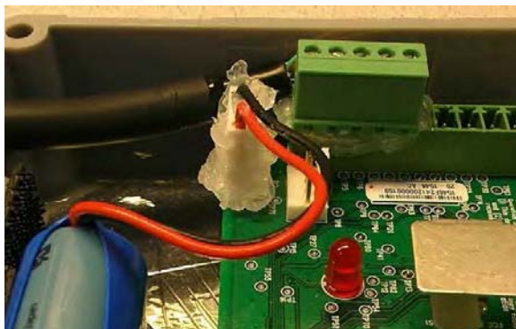
Figure 13 - 6. The Compound Must Cover Wires and Connectors for Watertight Seal
