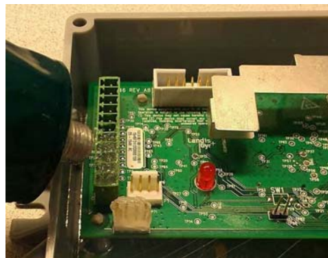
Figure 13 - 3. Apply the Compound to the GPR Pulse Input Connector
