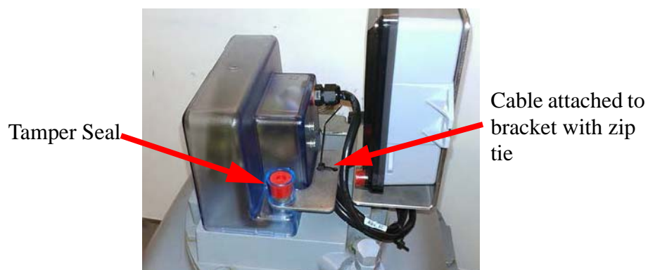
Figure 15 - 8. Attach Cable to Bracket with Black Zip Tie
