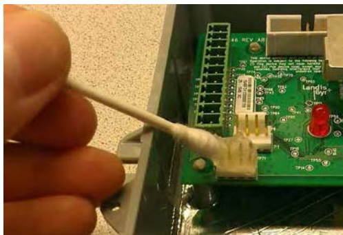
Figure 10 - 5. Force the Compound between Connector Pins
