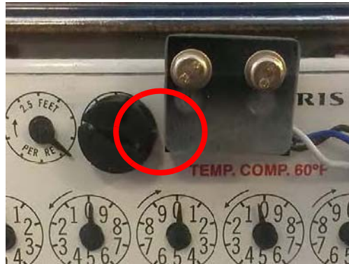
Figure 17 - 10. Gap Must Be Visible Between Wheel and Switch
