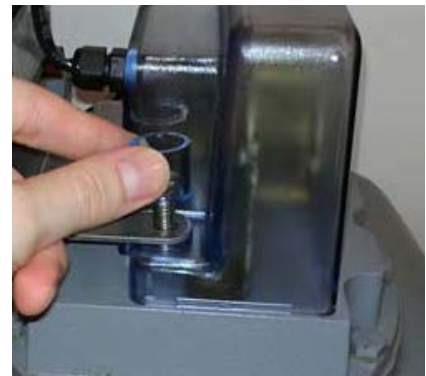
Figure 15 - 4. Install GPR Bracket, Screws and Tamper Cups
