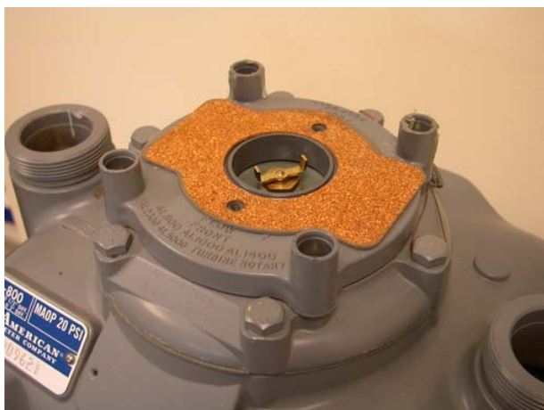
Figure 2 - 2. Base Plate with Tamper Seal Towers
