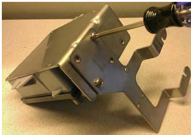
Figure A - 5. GPR Bracket Disassembly
