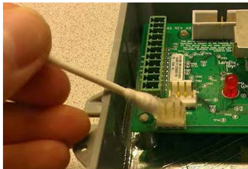
Figure 12 - 4. Force the Compound between Connector Pins
