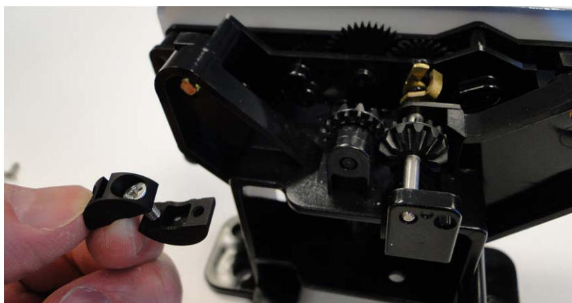
Figure 8 - 4. Slide Threaded Wheel Half Beneath the Index Drive Shaft
