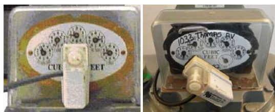
Figure 3 - 3. Center Dial and Offset Dial Mount Rockwell Commercial Index Covers
