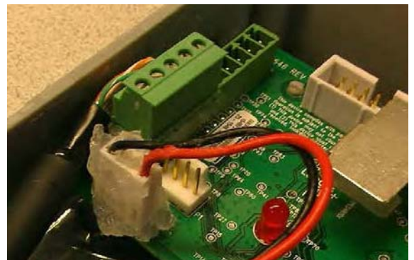
Figure 13 - 6. The Compound Must Cover Wires and Connectors for Watertight Seal
