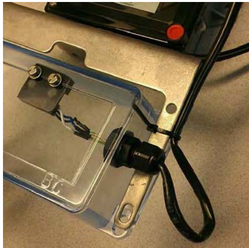
Figure 17 - 4. Switch Cover and GPR Assembly, with drip loop
