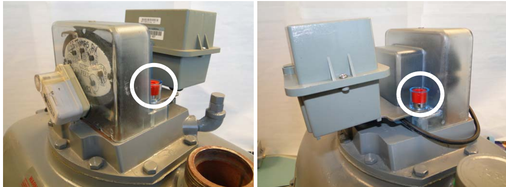
Figure 3 - 4. Remove Module Bracket Tamper Seals, Screws, and Gas Module Assembly
