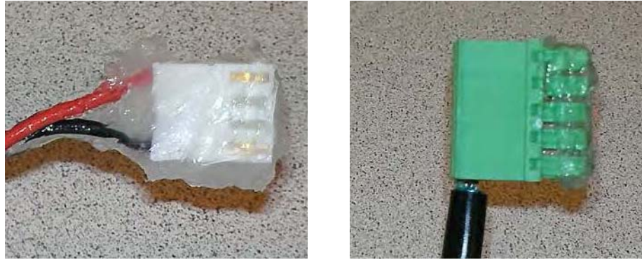
Figure 12 - 5. Apply the Compound to GPR Cable Connectors: Cover All Contacts
