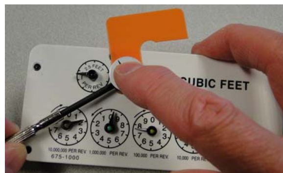
Figure 9 - 11. Tighten Pulse Wheel Screws to 1.2 \pm 0.10 Inch-Pounds
