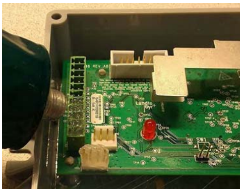
Figure 11 - 4. Apply the Compound to the GPR Pulse Input Connector
