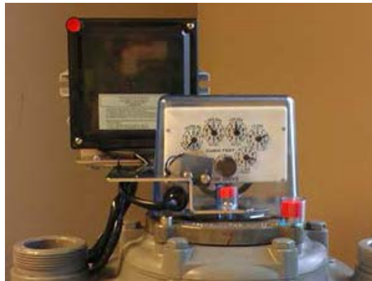
Figure A - 1. GPR at Left Rear - Using 28-1443 Bracket
