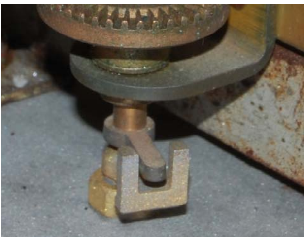
Figure 7 - 5. Index Drive Shaft Arm Alignment
