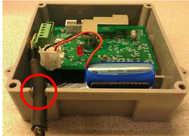
Figure 15 - 1. Pulse Interface Cable's Shrink Tubing Must Route Through GPR Strain Relief Slot
