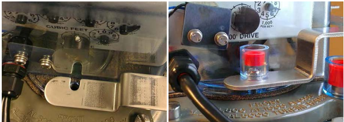
Figure 14 - 4. Tighten Front and Rear Cover Screws to 20 in-lbs ( \pm 5 in-lbs)
