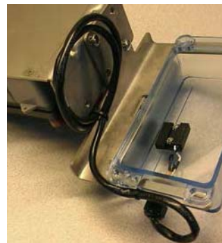
Figure 17 - 5. Excess Coiled Cable Attached Beneath GPR Bracket
