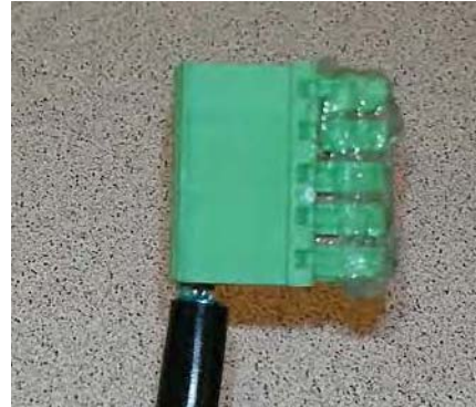
Figure 13 - 5. Apply the Compound to GPR Cable Connectors: Cover All Contacts
