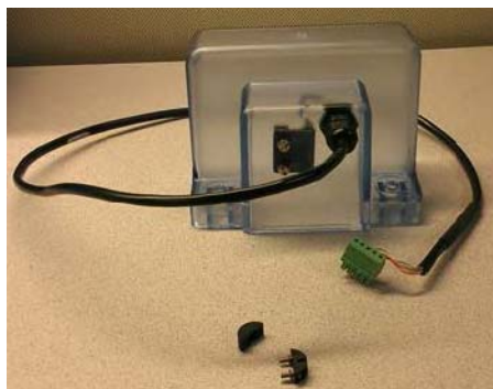
Figure 1 - 7. Solid State Pulser Index Cover and Magnet Wheel
