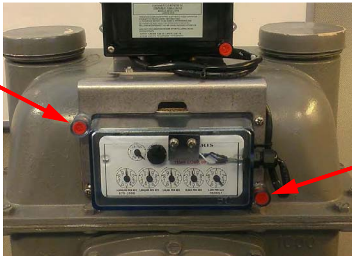
Figure 17 - 11. GPR Assembly installed on a Sprague Large Diaphragm Meter
