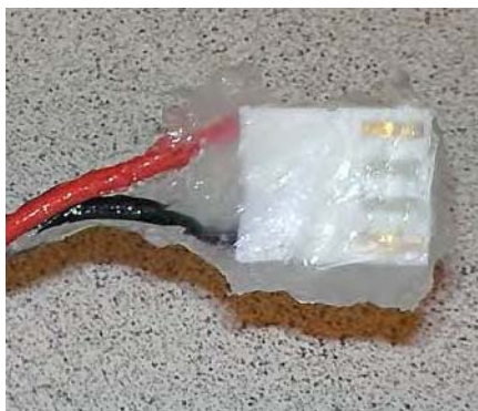
Figure 10 - 6. Apply the Compound to GPR Cable Connectors: Cover All Contacts
