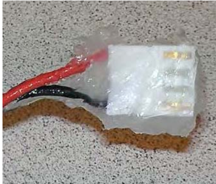
Figure 13 - 5. Apply the Compound to GPR Cable Connectors: Cover All Contacts
