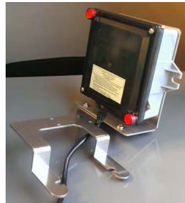
Figure A - 1. GPR at Left Rear - Using 28-1443 Bracket
