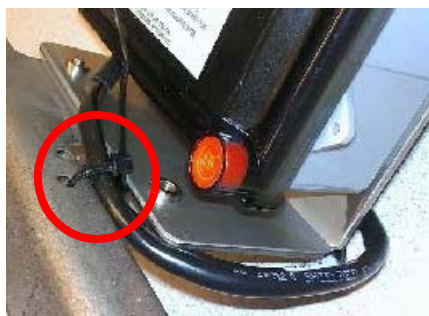
Figure 17 - 6. Excess Coiled Cable Attached Beneath GPR Bracket
