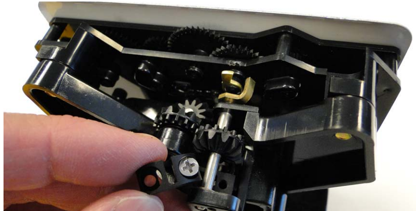
Figure 8 - 5. Slide Threaded Wheel Half Beneath Shaft
