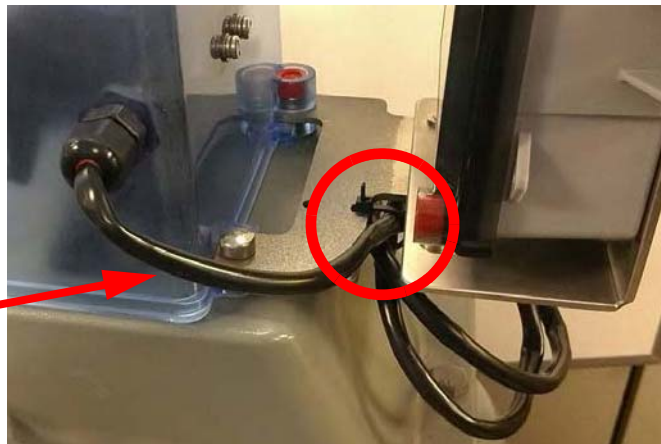
Figure 16 - 6. Route and Attach the Excess Cable
