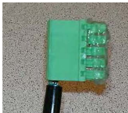
Figure 11 - 6. Apply the Compound to GPR Cable Connectors: Cover All Contacts
