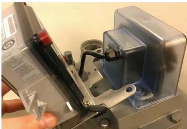
Figure 15 - 4. Install GPR Bracket, Screws and Tamper Cups
