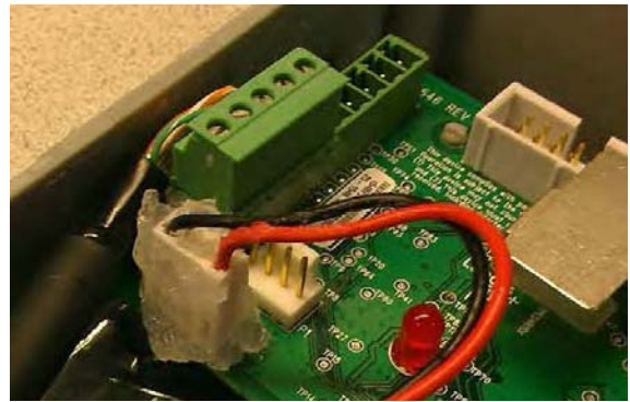
Figure 11 - 7. The Compound Must Cover Wires and Connectors for Watertight Seal
