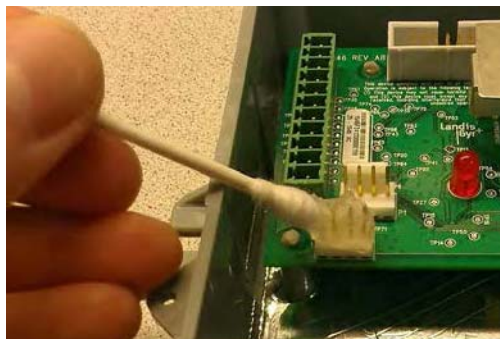
Figure 13 - 4. Force the Compound between Connector Pins
