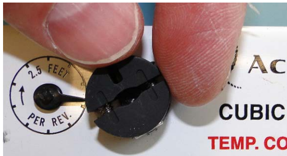
Figure 9 - 7. Pulse Wheel Must Not Contact Adjacent Pointers As It Rotates
