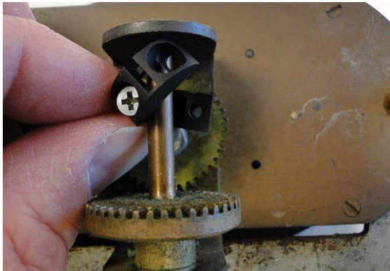
Figure 7 - 3. Place the Screw-bearing Notched Wheel Around the Index Drive Shaft
