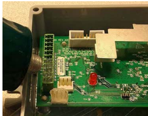
Figure 12 - 3. Apply the Compound to the GPR Pulse Input Connector
