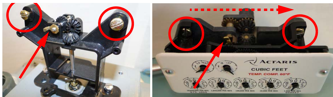
Figure 8 - 1. Index Screw and Drive Details
