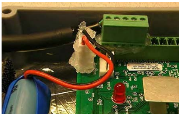
Figure 12 - 6. The Compound Must Cover Wires and Connectors for Watertight Seal
