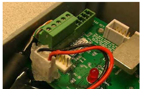
Figure 12 - 6. The Compound Must Cover Wires and Connectors for Watertight Seal
