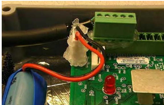
Figure 11 - 7. The Compound Must Cover Wires and Connectors for Watertight Seal
