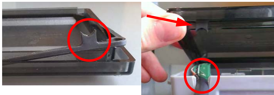
Figure 17 - 2. GPR Cover Gasket Tab and Cover Strain Relief Slot
