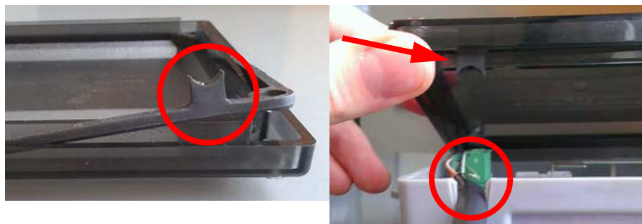
Figure 16 - 2. GPR Cover Gasket Tab and Cover Strain Relief Slot
