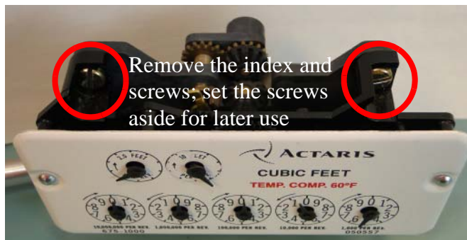
Figure 4 - 3. Remove Index and Screws; Discard the Unsupported Bracket Assembly
