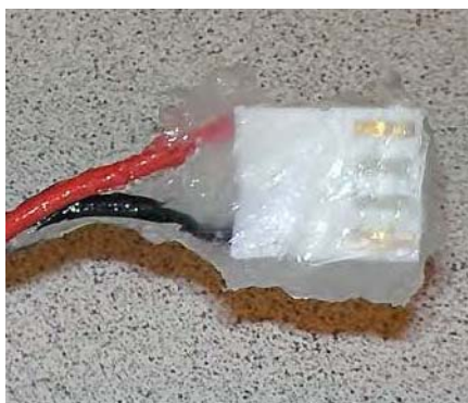
Figure 11 - 6. Apply the Compound to GPR Cable Connectors: Cover All Contacts
