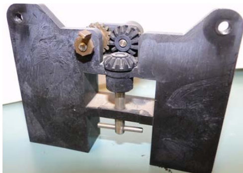
Figure 4 - 4. Index Removed from Unsupported Bracket Assembly
