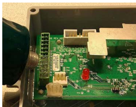
Figure 10 - 4. Apply the Compound to the GPR Pulse Input Connector
