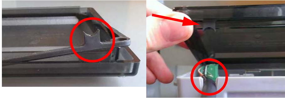
Figure 14 - 2. GPR Cover Gasket Tab and Cover Strain Relief Slot
