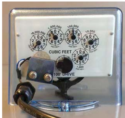
Figure 6 - 18. Dual Set-Screw Wheel on Plastic Pointer Index
