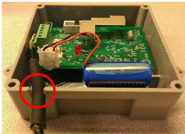
Figure 16 - 1. Pulse Interface Cable's Shrink Tubing Must Route Through GPR Strain Relief Slot
