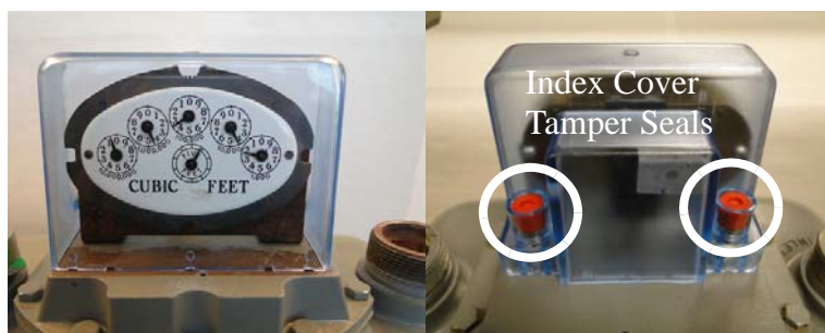
Figure 3 - 2. Remove Index Cover Tamper Seals, Screws, and Index Cover
