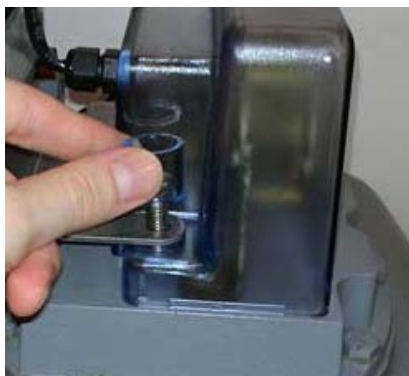
Figure 15 - 5. Tighten Bracket Screws 15 to 20 inch-pounds
