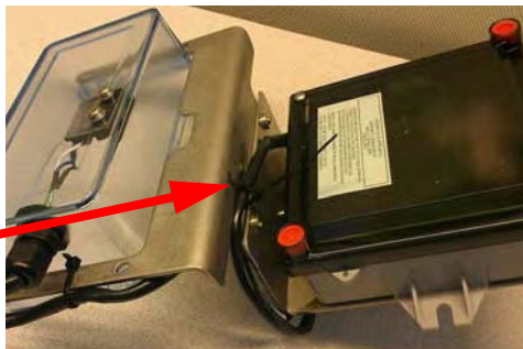
Figure 17 - 5. Excess Coiled Cable Attached Beneath GPR Bracket
