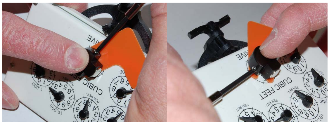
Figure 6 - 11. Tighten Pulse Wheel Screws to 1.20 inch-pounds ( \pm 0.10 inch-pound)
