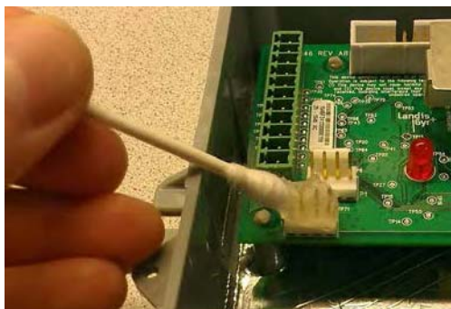
Figure 11 - 5. Force the Compound between Connector Pins
