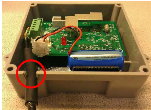
Figure 17 - 1. Pulse Interface Cable's Shrink Tubing Must Route Through GPR Strain Relief Slot
