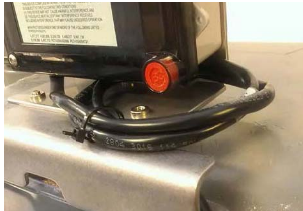
Figure 17 - 8. Cable Optionally Routed Above Index Cover Bracket
