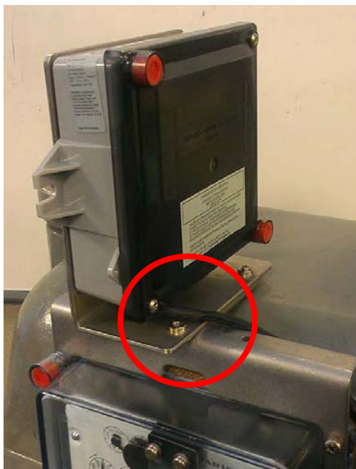
Figure D - 5. For Right-facing GPR Installs, Route Cable As Shown
