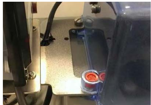
Figure 16 - 4. Slide Bracket into Index Cover Tamper Cup Slot
