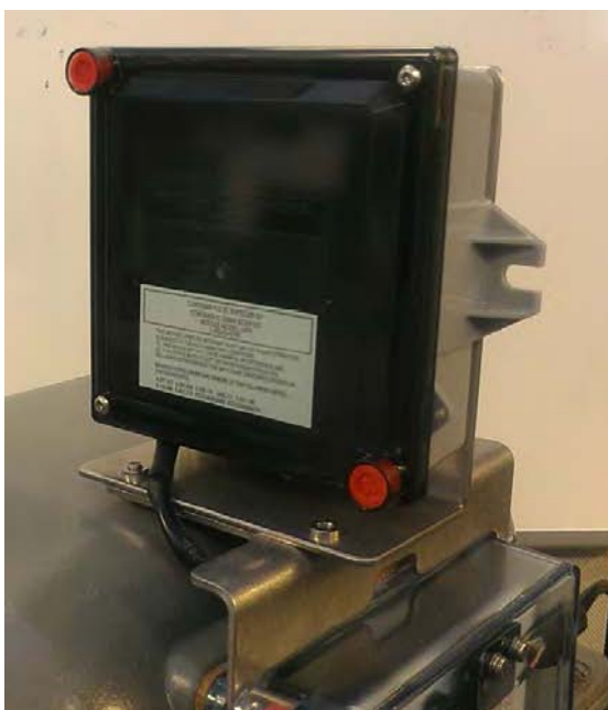
Figure D - 4. Left-Facing GPR Shown Extended Forward to Avoid Gas Pipe Interference
