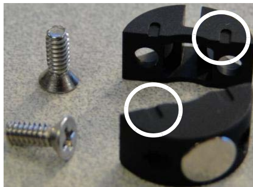
Figure 6 - 3. Where Alignment Slots Are Present On 2-Piece Magnetic Pulse Wheels, The Slots Must Be Installed On Top
