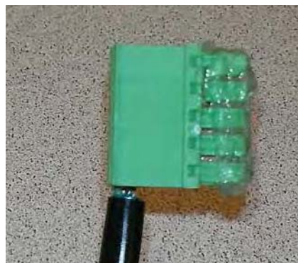
Figure 10 - 6. Apply the Compound to GPR Cable Connectors: Cover All Contacts
