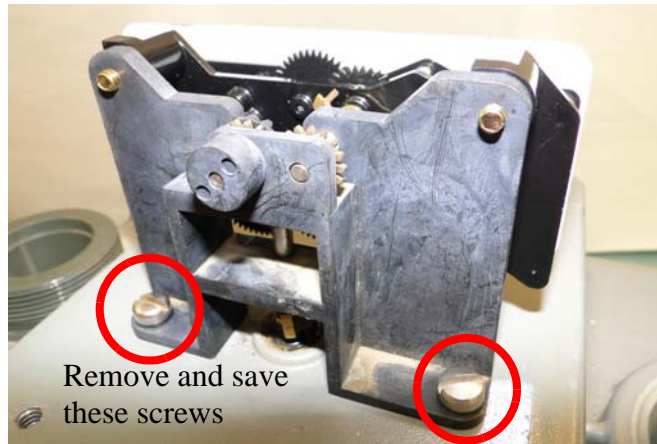
Figure 4 - 2. Unsupported Index Mounting Bracket Assembly
