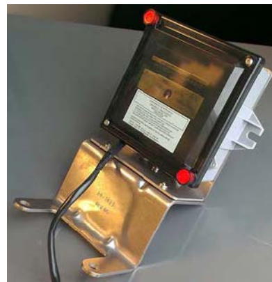
Figure A - 4. GPR at Center Rear - Using 28-1423 Bracket
