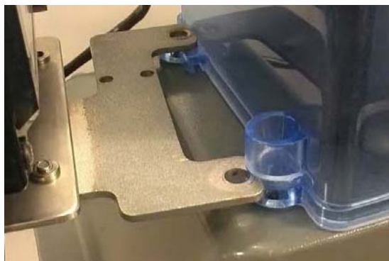
Figure 16 - 4. Slide Bracket into Index Cover Tamper Cup Slot
