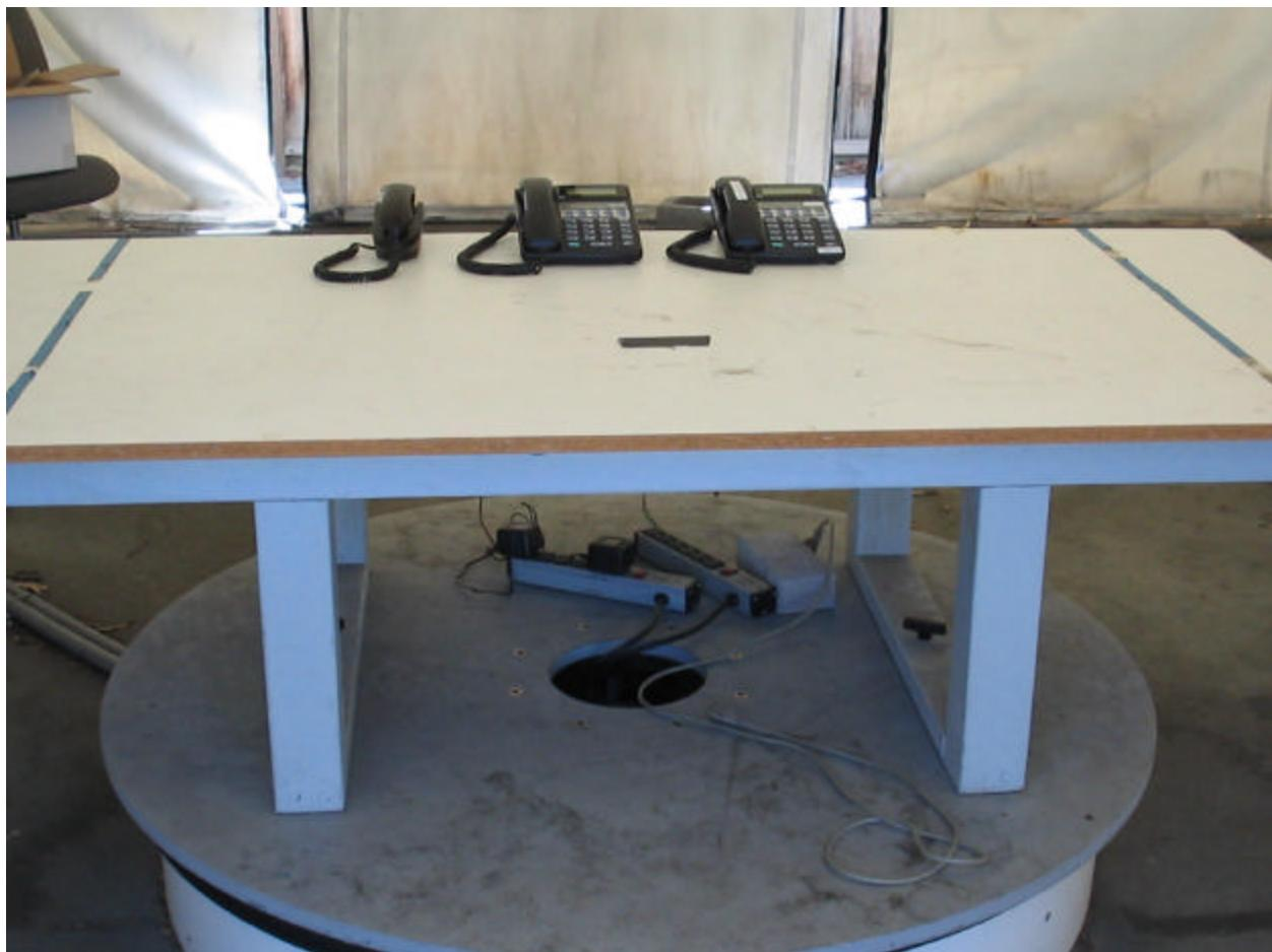
*Radiated Emissions Test Configuration Photographs*
