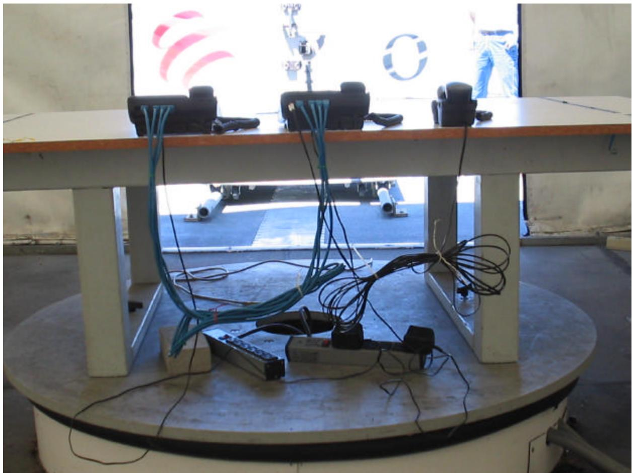
*Conducted Emissions Test Configuration Photographs*
