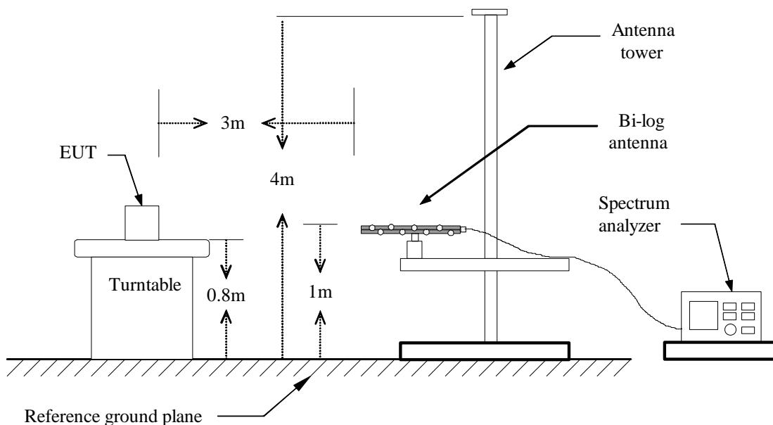
**Above 1 GHz**
