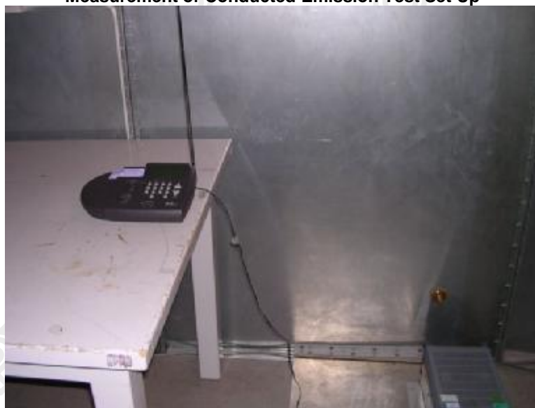
Measurement of Conducted Emission Test Set Up
