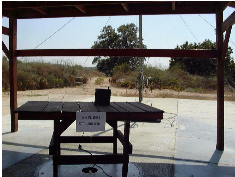
Figure 3. Out of Band Emission (Radiated) and Radiated Emission Part 15 Test Setup
