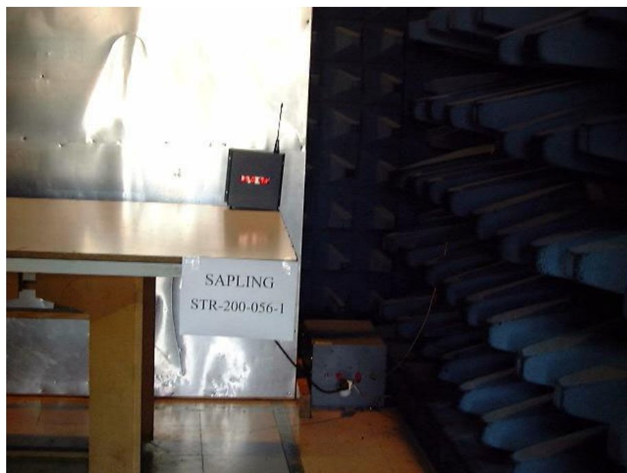
Figure 2. Conducted Emissions on AC Lines Test Setup
