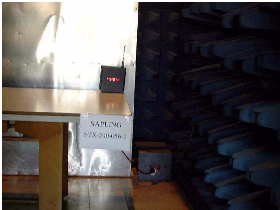
Figure 78. Conducted Emissions on AC Lines Test Setup
