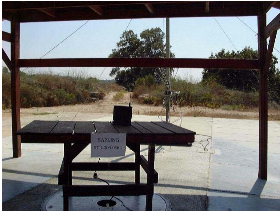
Figure 79. Out of Band Emission (Radiated) and Radiated Emission Part 15 Test Setup
