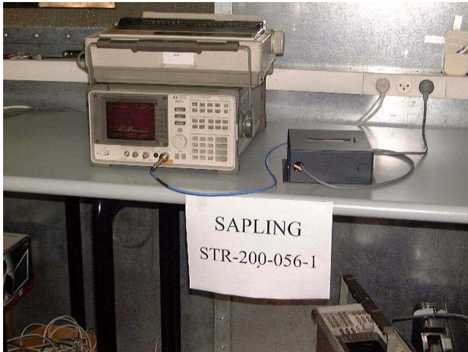
Figure 77. Emissions on Antenna Ports Test Setup
