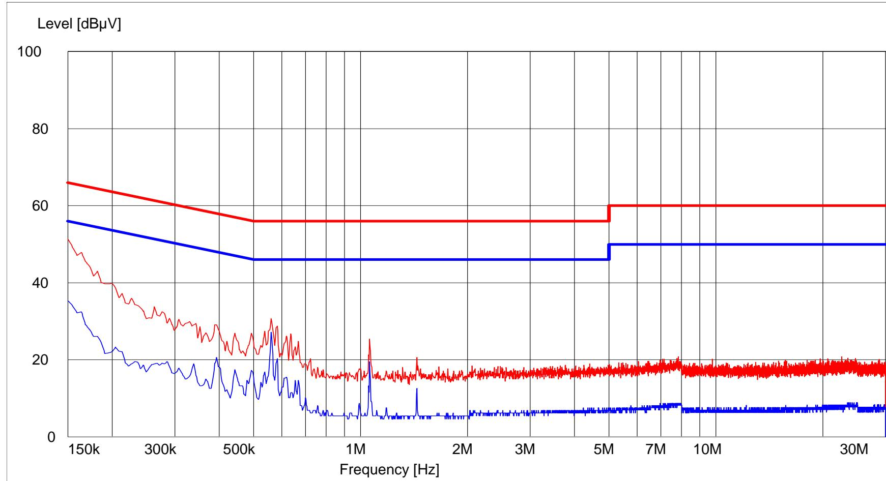
FCC 15.207 Conducted Emissions 150kHz to 30MHz
