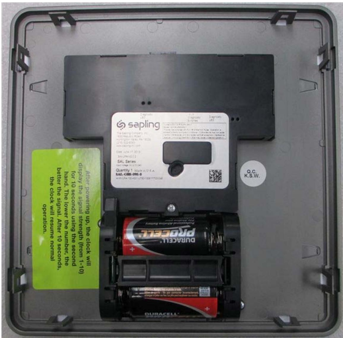
After powering up, the clock will display the signal strength (from 1-10) for 10 seconds using the second hand. The lower the number, the better the signal. After 10 seconds, the clock will resume normal operation.
