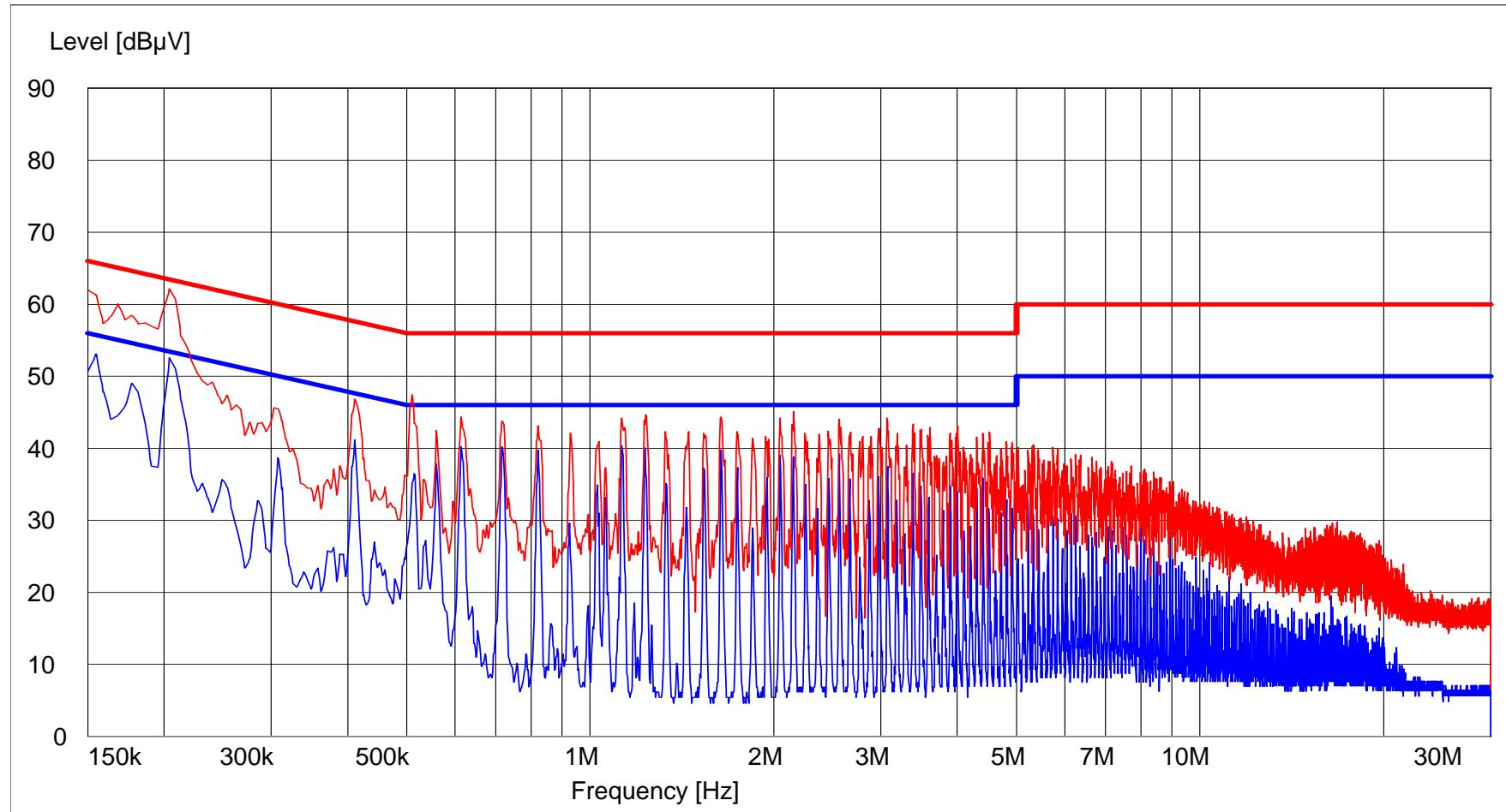
**FCC Part 15, Subpart C, Section 15.107(a), Conducted Emissions, Power Leads
