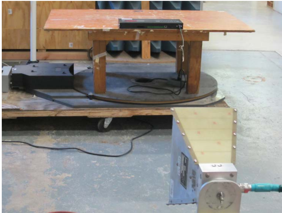
Master Clock, Horizontal Antenna Polarization
