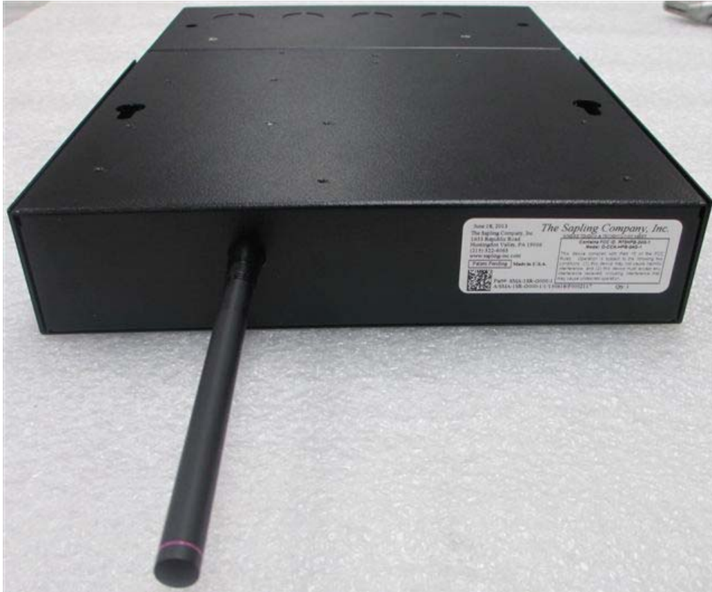
SMA-1SR-G000-1, Repeater Label Location
