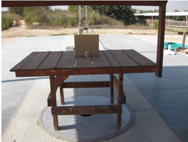
Figure 2. Open Site Radiated Emission Test
