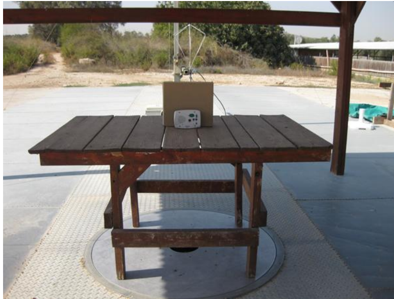
Figure 2. Open Site Radiated Emission Test
