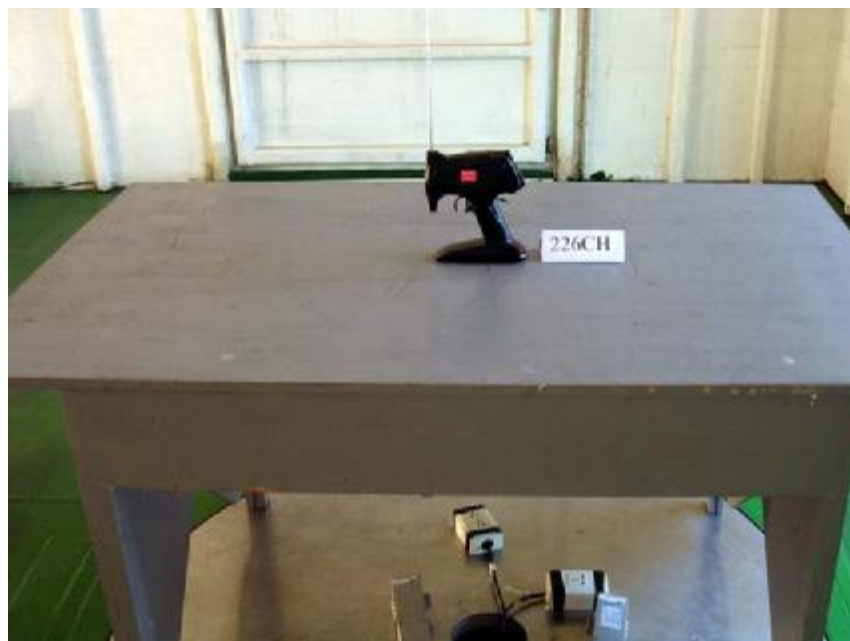
Photo 2: Radiated Emission Test Set-up
