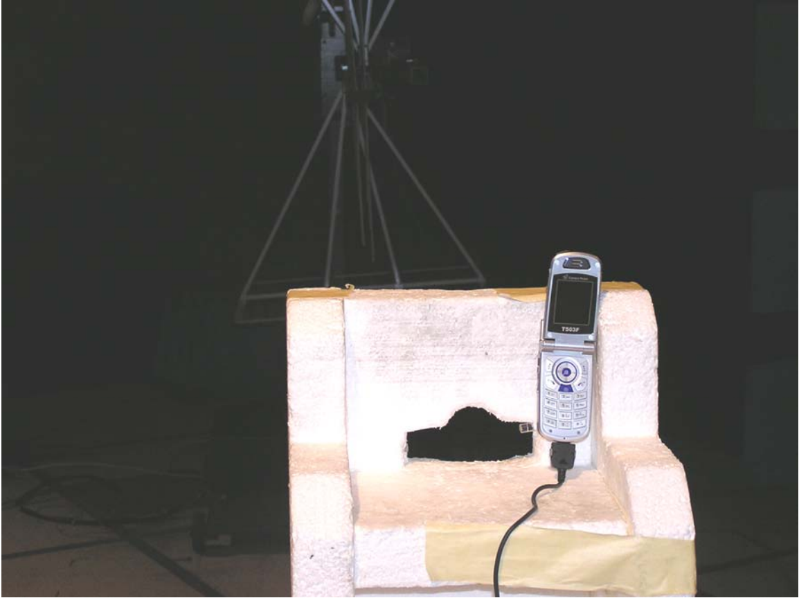
Test setup – Radiated Emissions
