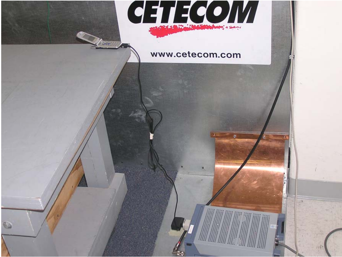
Test setup – AC Line Conducted Emissions
