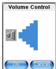
To adjust the earpiece volume, press the buttons on a side of the phone during a call. The display will briefly show your current volume setting.
