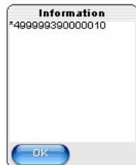
Every phone that is manufactured has a globally unique number which is used to identify it to the network. This number is known as your IMEI number and is independent of the details of your subscription with the network operator. This screen displays the IMEI number of your phone.
