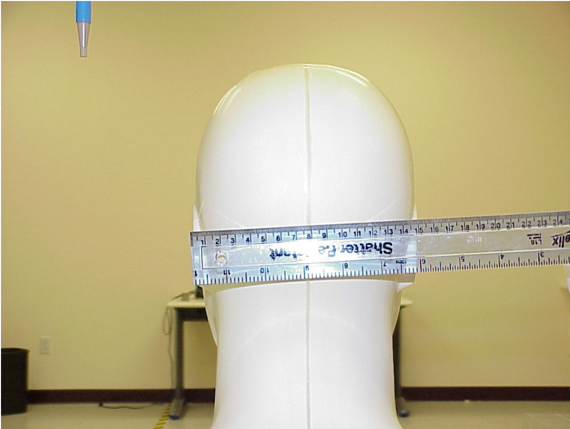
Photo 10. Photo to demonstrate 15 cm Z-axis head phantom
