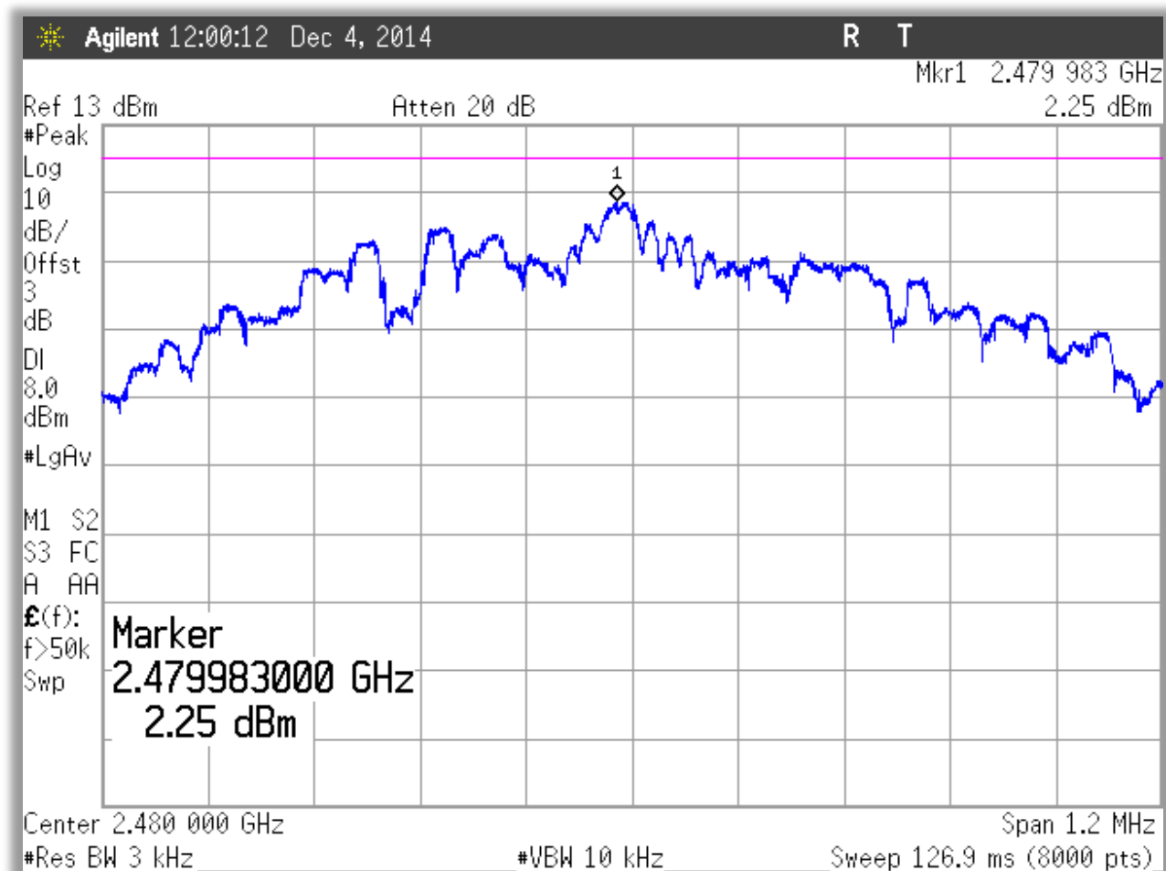
Figure 15: Power Spectral Density, High Channel - High Power Mode
